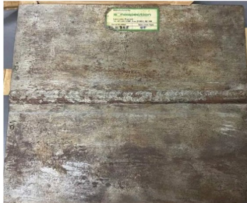
Fig. 2 Single Vee Butt Welded test specimen
