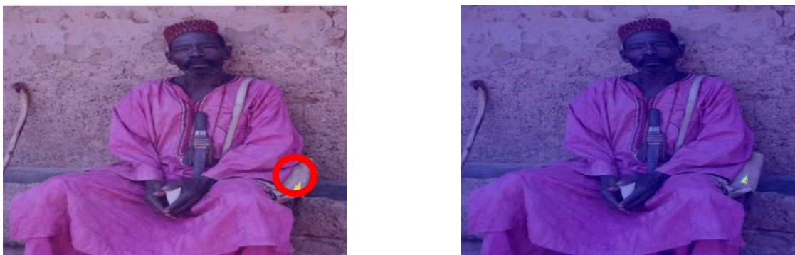
Fig. 4 (Left) The best-performing test image and the overlaid predicted map (yellow hue) with mean IU and DS of 0.93 and 0.88, respectively. (Right) The deConv layer feature activation map
