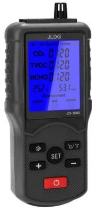
Fig. 3 (a) Multifunctional Air Quality Tester CO2 measuring device (Model JD-3002); (b) Handheld Digital Anemometer for air temperature, movement, and relative humidity
