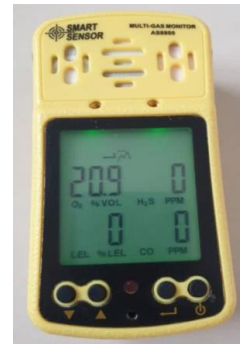
Fig. 2 Smart Sensor Multi Gas Monitor (Model AS8900) for CO and O2 measurements
