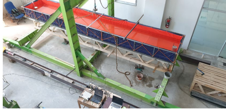
Fig. 10 Test situation of composite floor loaded by 300 mm water height
