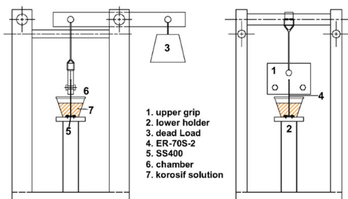
**Fig. 2** Jig and fixture for SCC test
