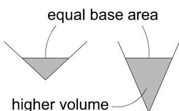
**Fig. 7** Higher available melting metal for sharper wire tip
