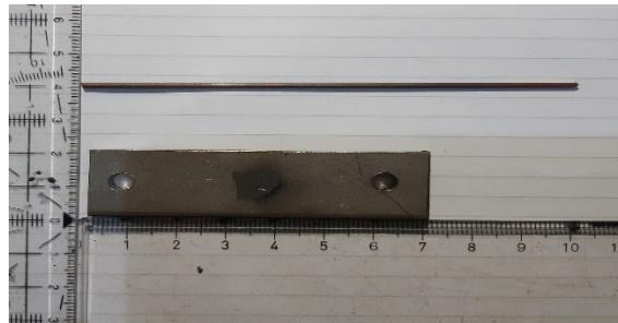
**Fig. 3** ER70S wire and SS400 plate**Table 3** Parameters of hotspot CDW
