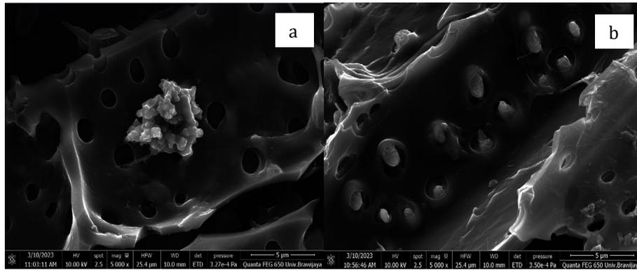
Fig. 5 SEM image of CA after the medical waste adsorption process (a) GA; (b) BV
