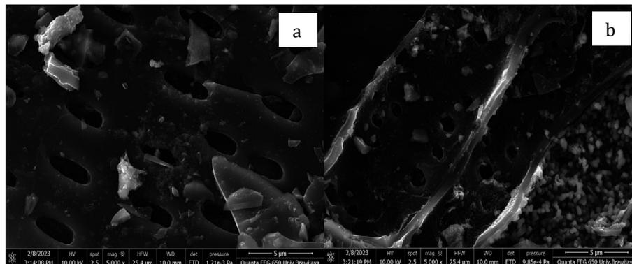
**Fig. 3** The scanning electron microscopy of bamboo charcoal (a) GA; (b) BV
