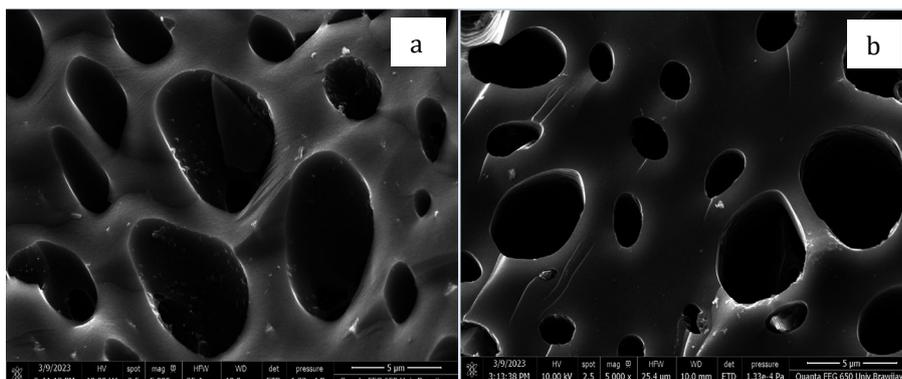
**Fig. 4** SEM of bamboo charcoal after activation with HCl (a) GA; (b) BV
