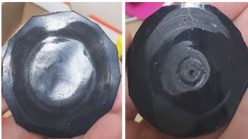
Fig. 11 A comparison between proper alignment on the left side and misalignment on the right side
