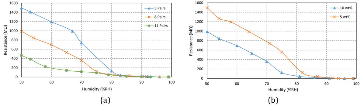
**Fig. 7** Sensor resistance for different (a) IDE electrode pairs; (b) PVA concentration
