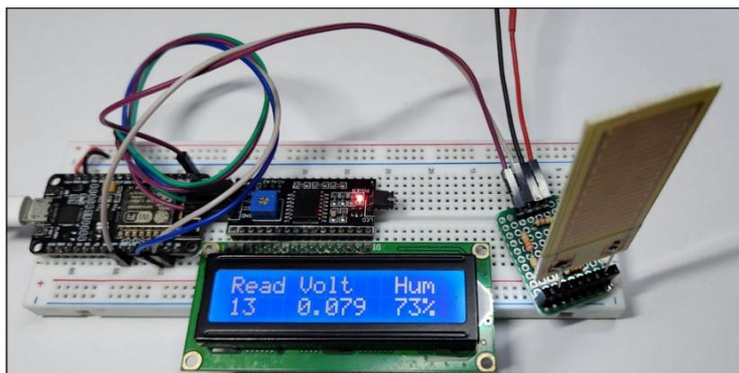
**Fig. 11** Final prototype measuring humidity at 73 %RH
