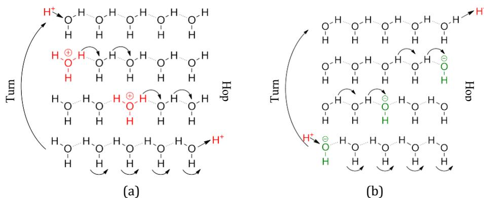
**Fig. 2** Hop and turn Grothuss mechanism for conductivity of (a)  $H^+$  as hydronium ion along proton wire; (b)  $OH^-$  as proton hole along proton wire [26]
