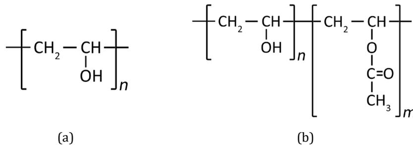
**Fig. 1** PVA structural formula representation for (a) fully hydrolysed; (b) partially hydrolysed PVA
