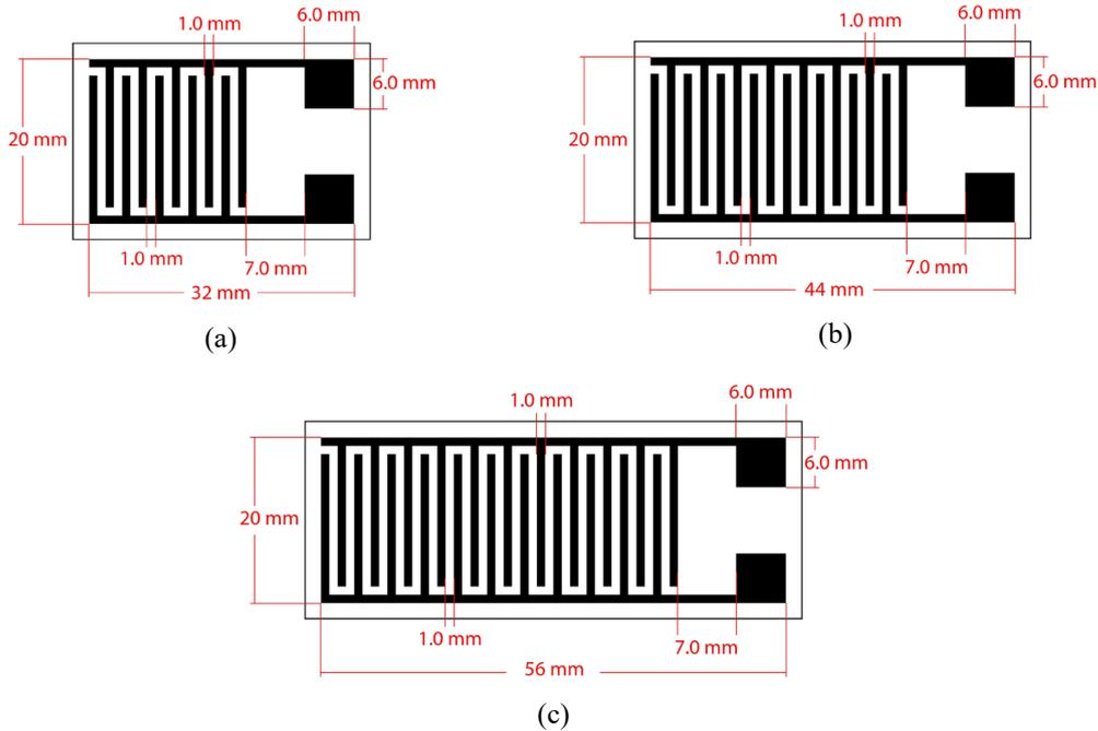
**Fig. 3** Interdigitated electrode layout with (a) 5 finger pairs; (b) 8 finger pairs; (c) 11 finger pairs
