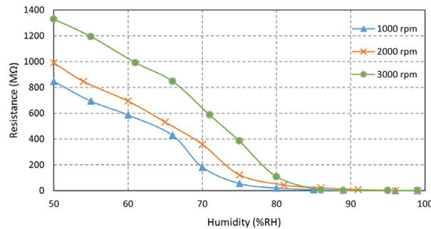
**Fig. 8** Sensor resistance for different spin coating speeds
