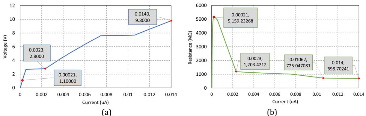
**Fig. 5** IV measurements interpreted in form of (a) Voltage vs. current; (b) Resistance vs. current
