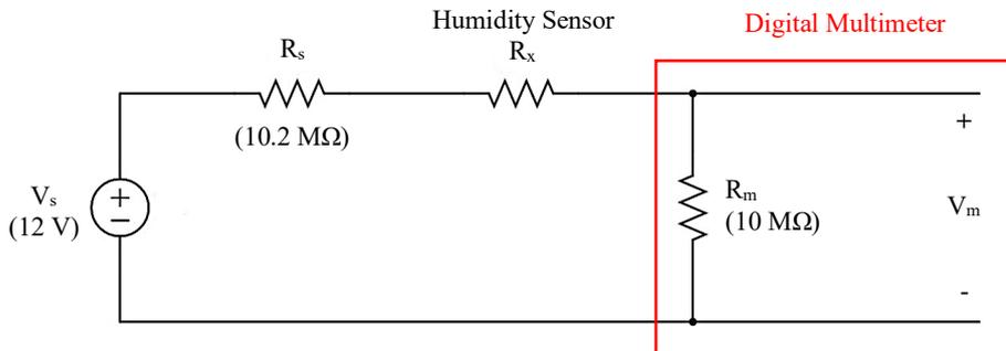
Fig. 6 Interface circuit used for resistance measurements
