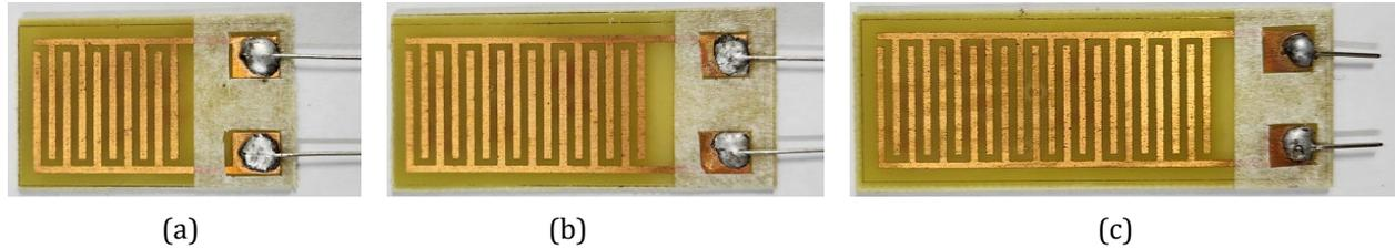
**Fig. 4** The fabricated humidity sensor with (a) 5 pairs; (b) 8 pairs; (c) 11 pairs of electrodes
