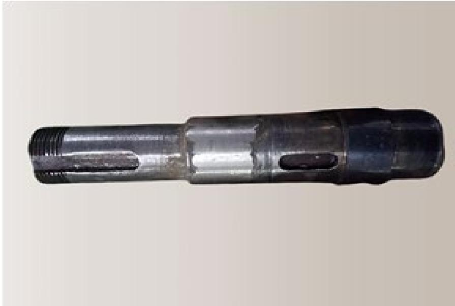
**Fig. 1** *The wear of the shaft timing pulley on the ring frame machine*
