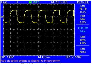
Fig.12 Inverter Output voltage.
