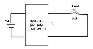
Fig.3 Average PWM Inverter Model.
