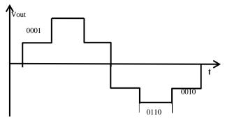
Fig. 2 Expected Result of Six Pulses Output Inverter Waveform.
