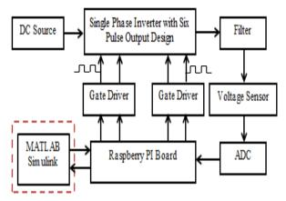
Fig.1 Block Diagram of the Project.
