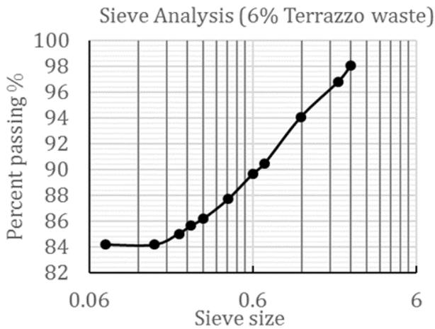
Fig.6 Sieve analysis for 6% admixture.
