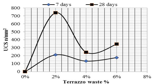
Fig.12. Variation of UCS values at 2, 4 and 6% admixed terrazzo waste for 7 and 28 days curing.
