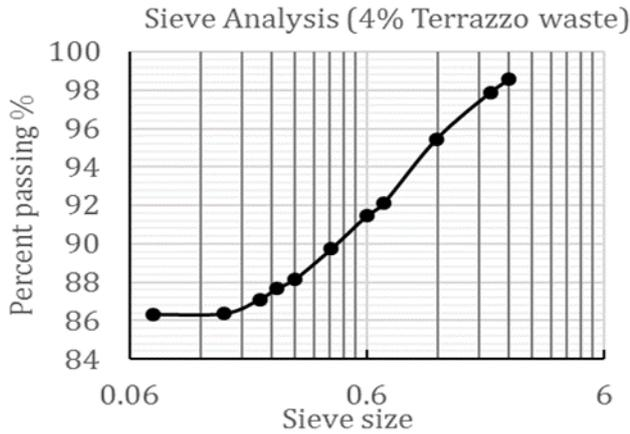
Fig.5 Sieve analysis for 4% admixture.
