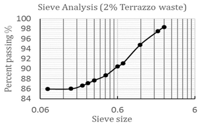
Fig.4 Sieve analysis for 2% admixture.
