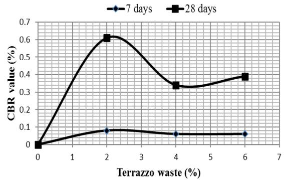
Fig.11. CBR values for 7 and 28 days soaked at 0, 2,4, and 6 % admixture.
