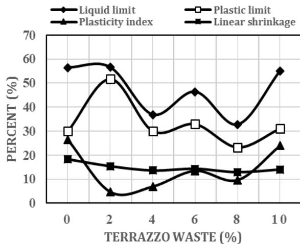
Fig.2 Atterberg limits for 0 - 10% admixture.
