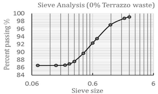
Fig.3 Sieve analysis for 0% admixture.
