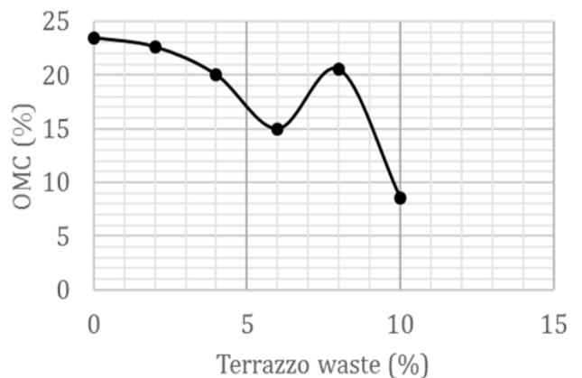
Fig.8 OMC optimums for 2 - 10% admixture.
