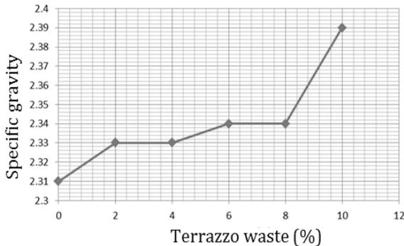
Fig.1 Effect of variation of terrazzo waste content on the specific gravity.
