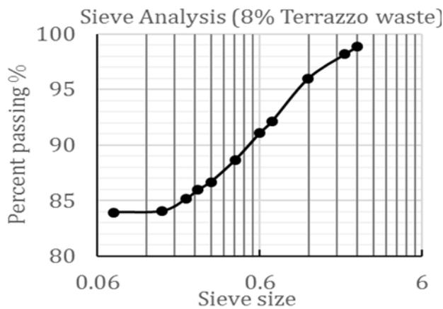
Fig.7 Sieve analysis for 8% admixture.
