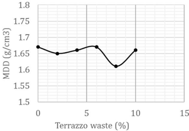
Fig.9 MDD optimums for 2 - 10% admixture.
