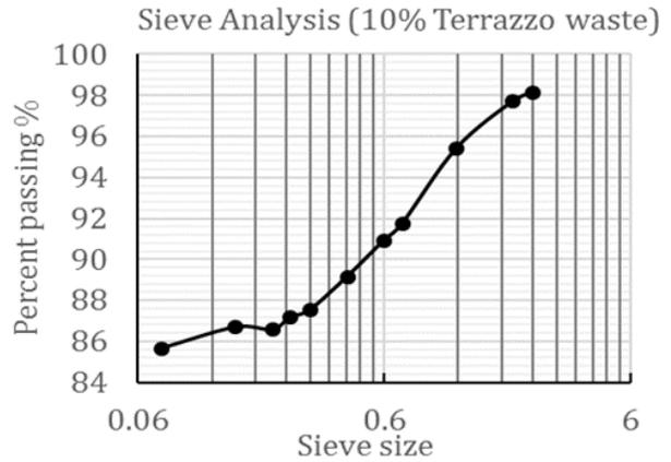
Fig.8 Sieve analysis for 10% admixture.
