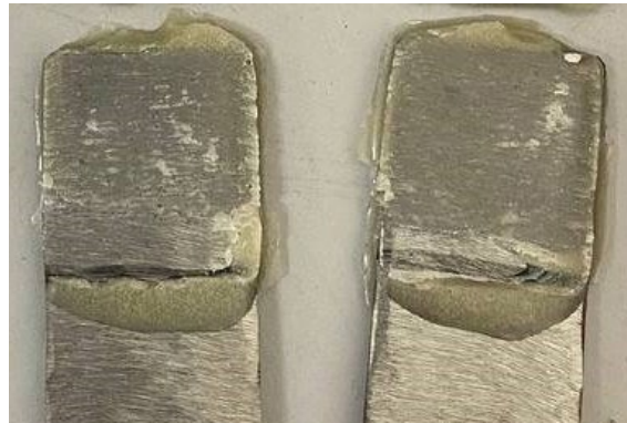
Fig. 9 Cohesive failure modes seen upon testing (taken from SLJ-5%-25.4mm overlap length)
