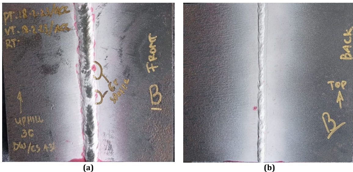
Fig. 7 (a) Penetrant interpretation surface area of specimen 2; (b) Penetrant interpretation root area of specimen 2
