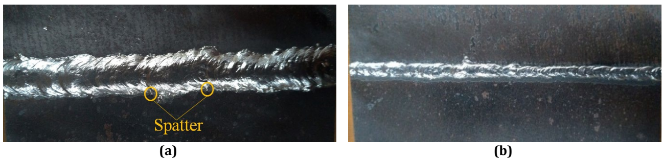
Fig. 5 (a) Visual weld surface area specimen 2; (b) Visual weld of the root area specimen 2
