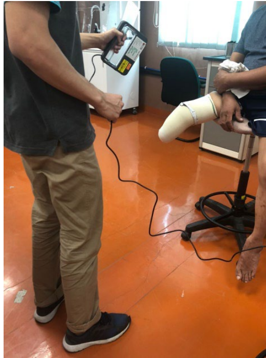
Fig. 1 Three-dimensional scanning of patient's residual leg
