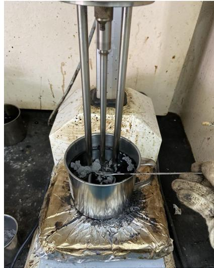
Fig. 2 - Silverson mechanical mixture
