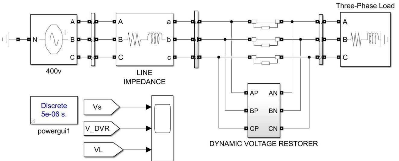
**Fig. 4 - 400V distribution system with dynamic voltage restorer MATLAB Simulink model**
