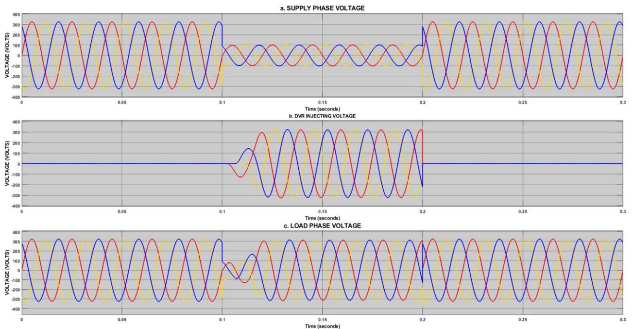
**Fig. 8 - Voltage waveforms with DVR (a) supply phase voltage; (b) DVR injecting voltage; (c) load phase voltage**
