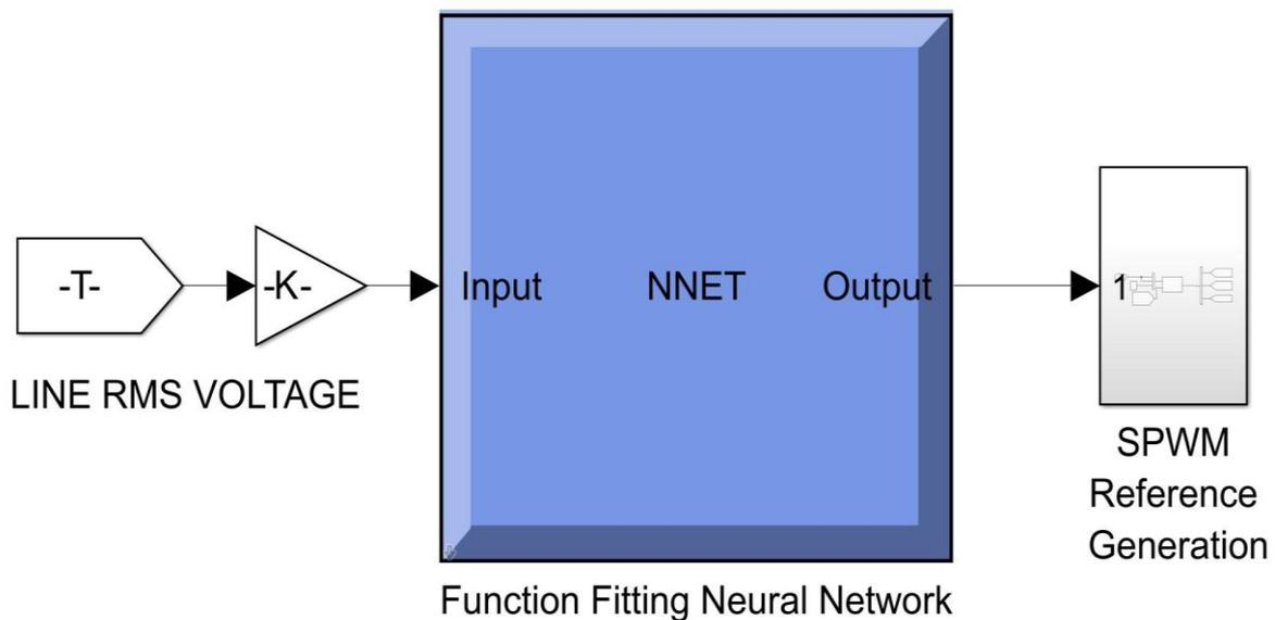
Fig. 6 - Artificial neural network controller
