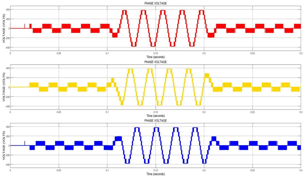
**Fig. 9 - Cascade H-Bridge multilevel inverter 9-Level voltage waveforms**
