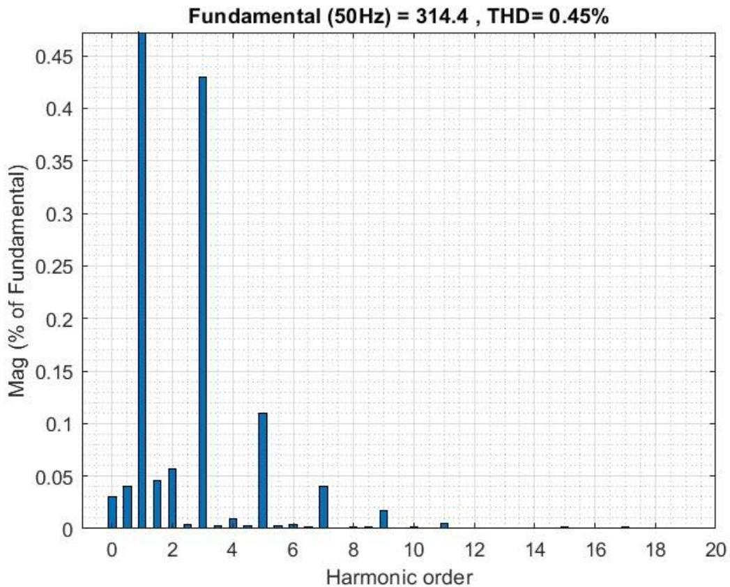
Fig. 12 - THD analysis of load phase voltage
