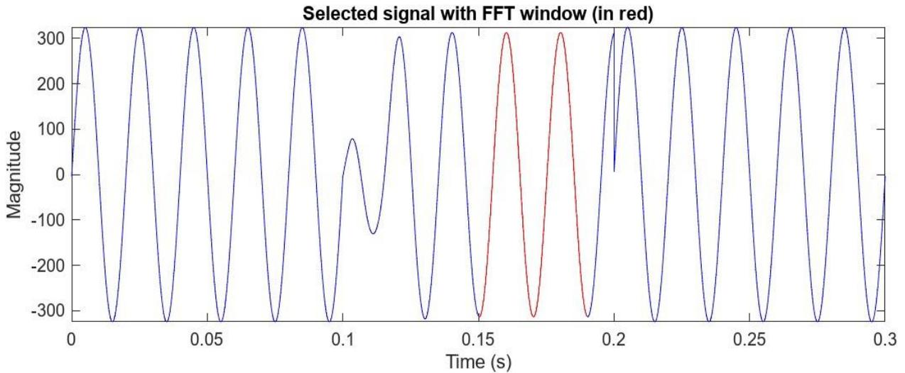
Fig. 11 - Load phase voltage for THD analysis
