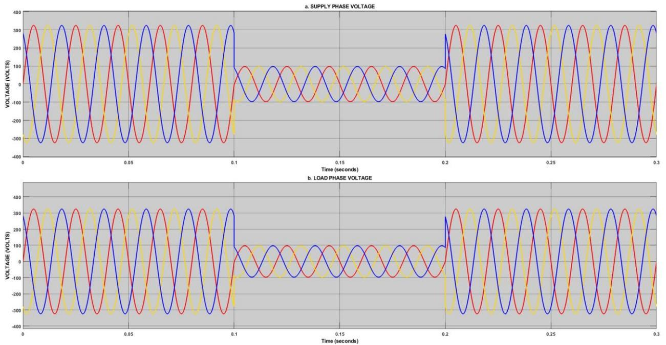
**Fig. 7 - Voltage waveforms without DVR (a) supply phase voltage; (b) load phase voltage**
