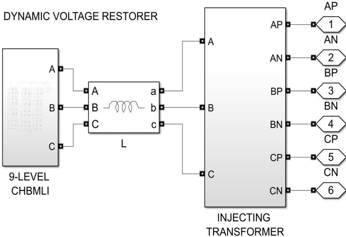
Fig. 5 - Dynamic voltage restorer MATLAB Simulink model
