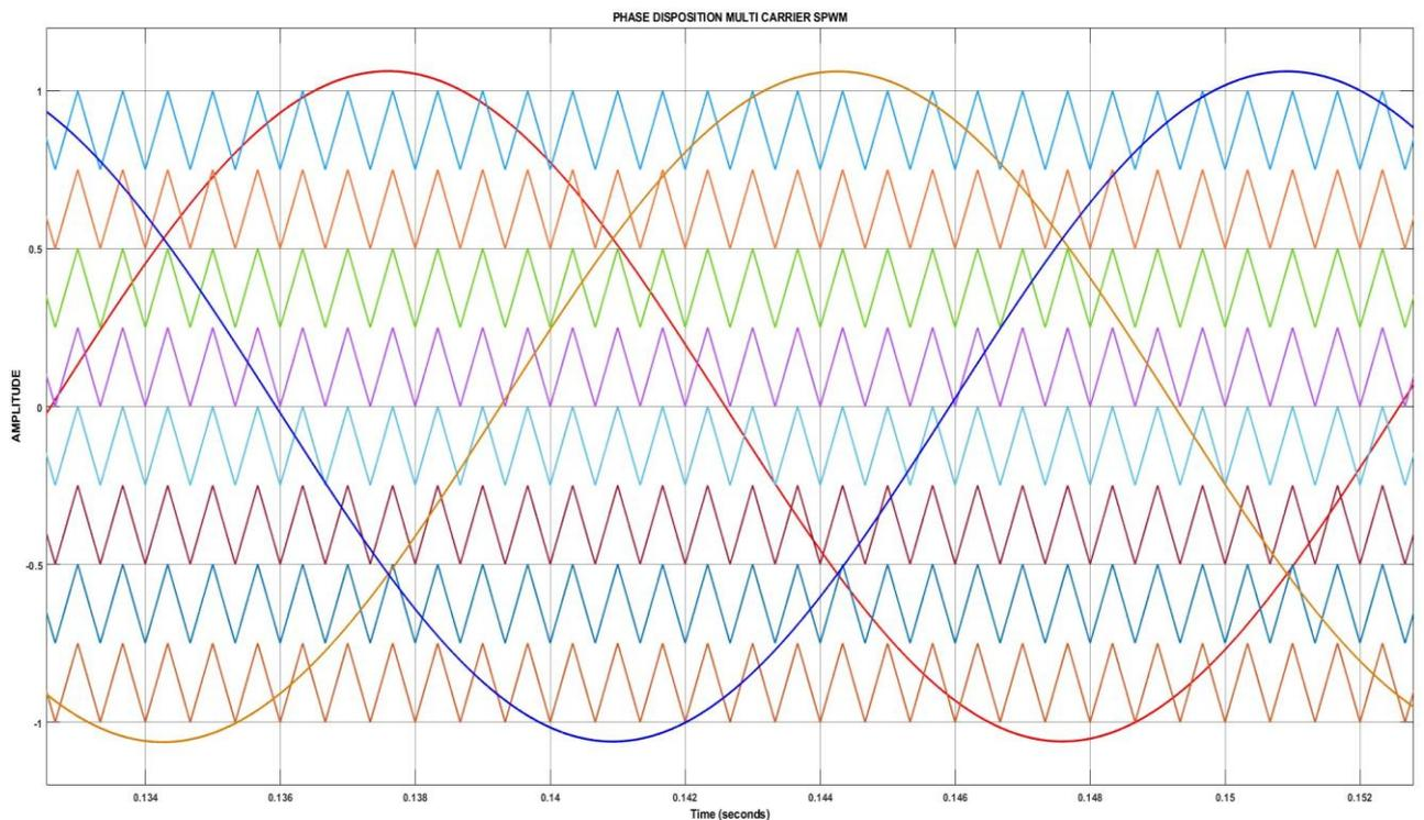
**Fig. 10 - Cascade H-Bridge multilevel inverter phase disposition multi carrier SPWM**
