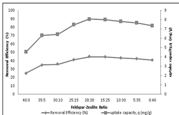
Fig. 1 The optimum ratio of Feldspar-Zeolite for COD removal at pH 7 and 200 rpm shaking speed
