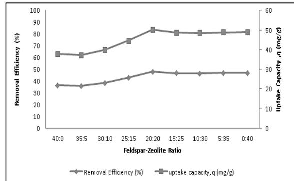
Fig. 2 The optimum ratio of Feldspar-Zeolite for NH<sub>3</sub>-N removal at pH 7 and 200 rpm shaking speed
