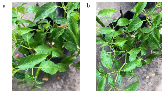
Fig. 8 - Pesticide coverage quality on top side (a) 2 seconds; (b) 3 seconds of spraying time
