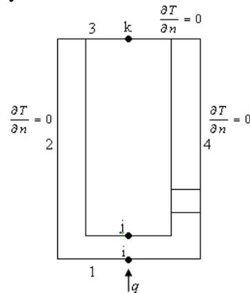
Fig. 2 Electrode heat flux with boundary conditions.
