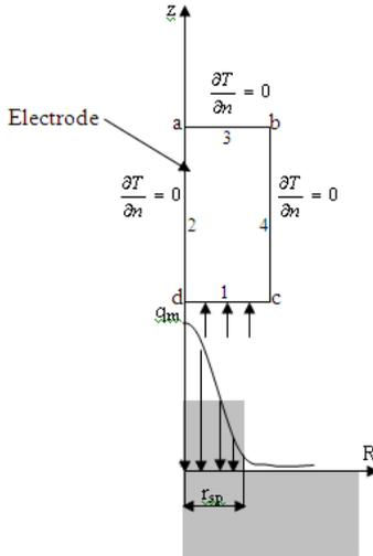
Fig. 1. Gaussian heat distribution for modeling the electrode.
