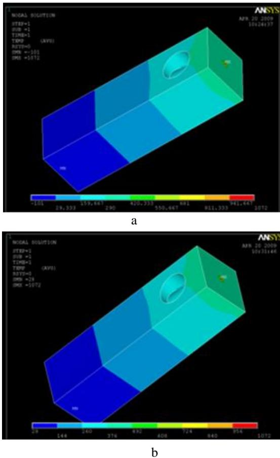
Fig. 3 Variations in temperature distributions on the electrode: (a) EDM with nitrogen, (b) EDM without nitrogen.
