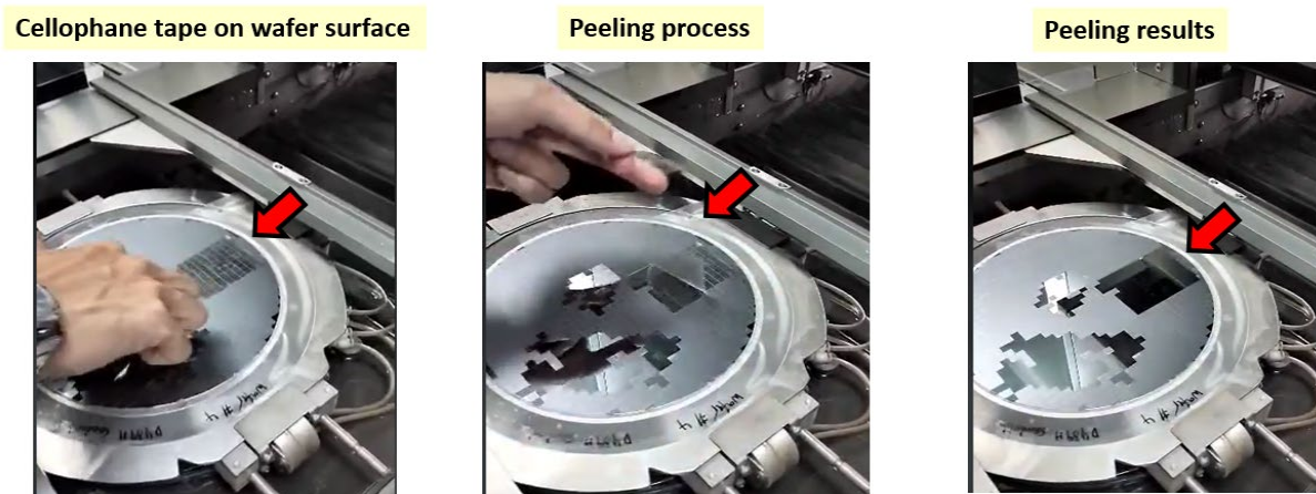
Fig. 2 Surface mounting peeling process on dicing chuck table
