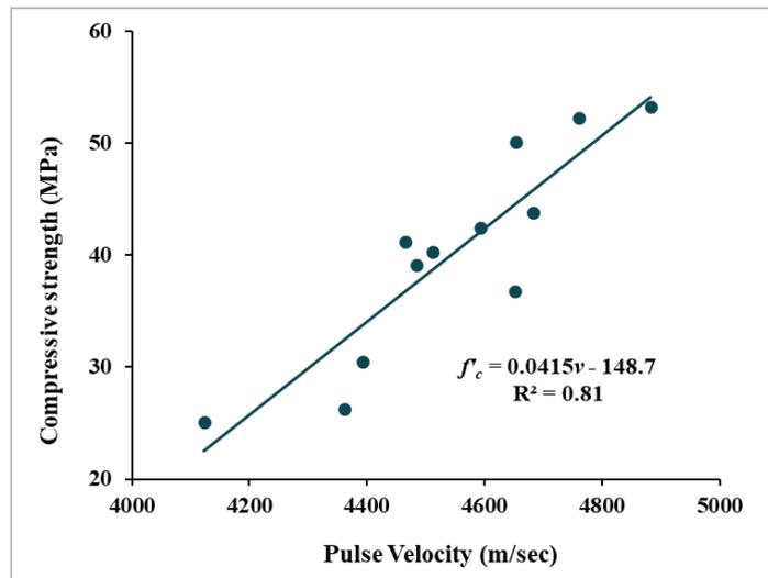
**Fig. 6 - Relationship between destructive compressive strength and pulse velocity**
