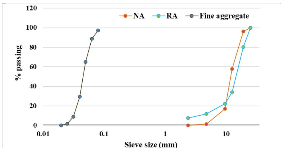
Fig. 1 - Particle size distribution of normal, recycled, and fine aggregate
