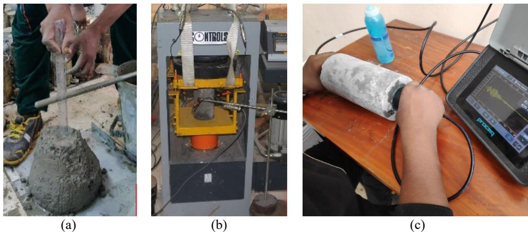
Fig. 2 - Experimental set-up (a) slump test; (b) compressive strength, and; (c) UPV test
