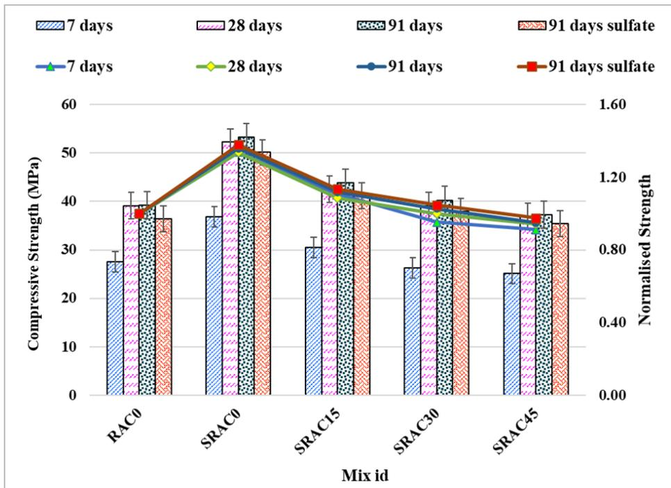
Fig. 4 - Compressive strength and normalized strength, along with the mix id
