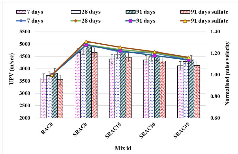
Fig. 5 - UPV and normalised pulse velocity along with the mix id
