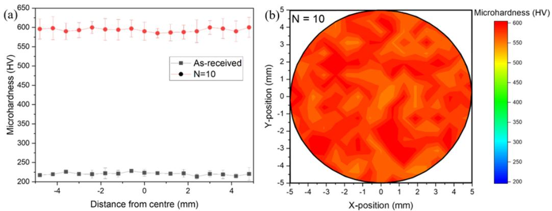
**Fig. 2** HV measurements (a) across the diameter; and (b) throughout the surface of the as-received and HPT-processed disks
