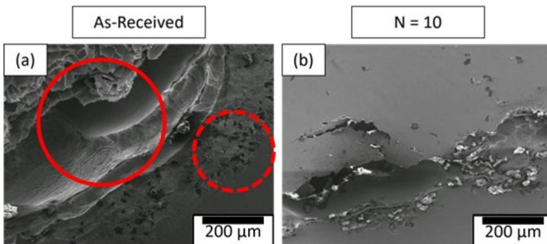
**Fig. 4** Representative SEM images of the worn samples (a) before HPT processing; and (b) after 10 HPT revolutions
