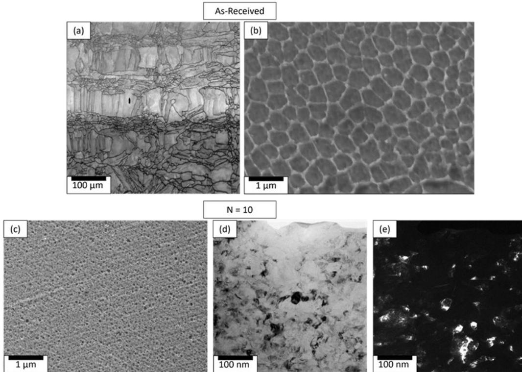
**Fig. 1** Microstructures of as-received samples (a) and (b); and microstructures after 10 HPT revolutions (c) – (e)
