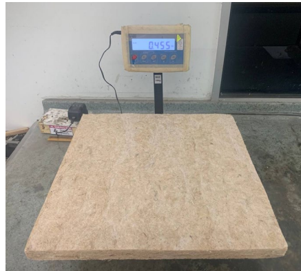
Fig. 2 Non-woven kenaf fibre by-product provided by the National Kenaf and Tobacco Board (NKTB)
