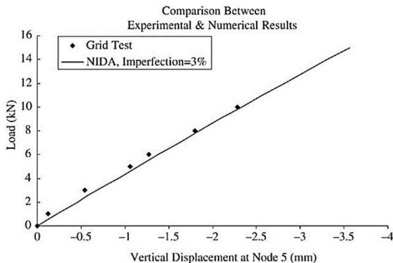
Fig. 7 - Load-displacement diagram of bamboo truss with PVC joint material [19]
