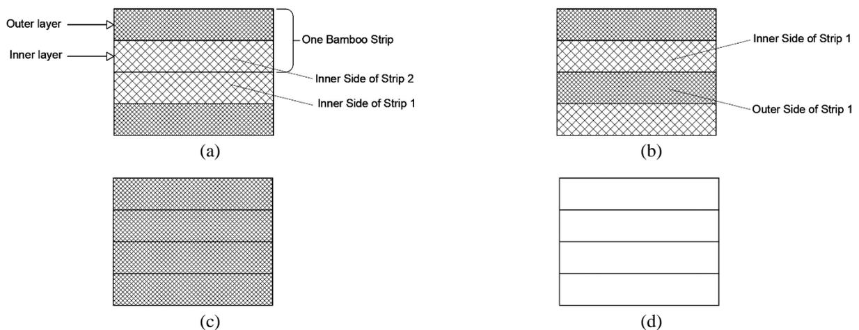
Fig. 3 - Different configurations of layered bamboo strips [21]
