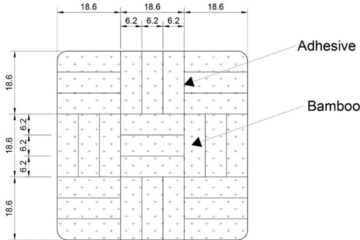
Fig. 2 - Cross-section of glubam truss member [18]
