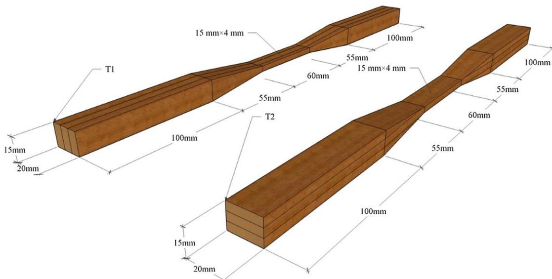
**Fig. 4 - Dog-bone-shaped bamboo strip for tensile strength test [18]**
