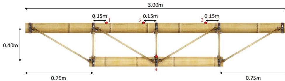
Fig. 9 - Sample bamboo truss made from *Guada angustifolia* [26]
