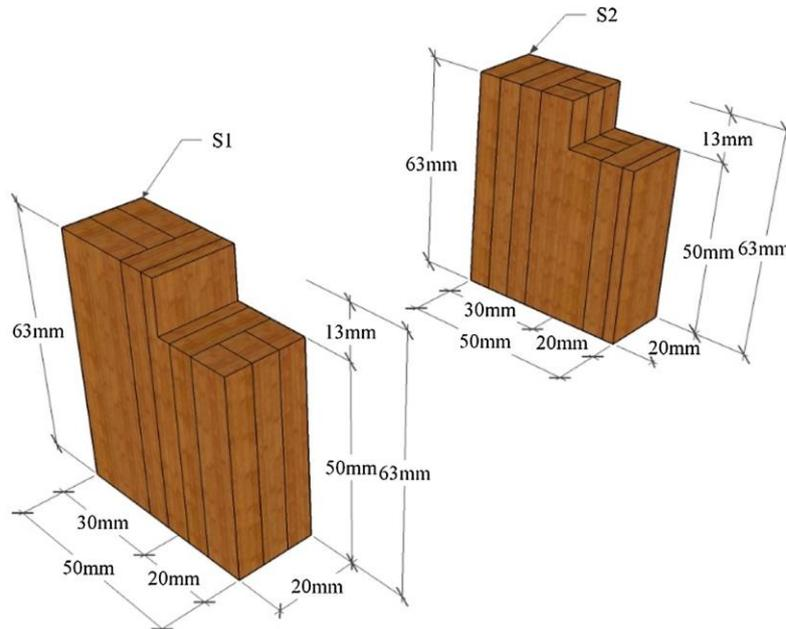
**Fig. 5 - Shape and size of bamboo specimen for shearing strength test [18]**
