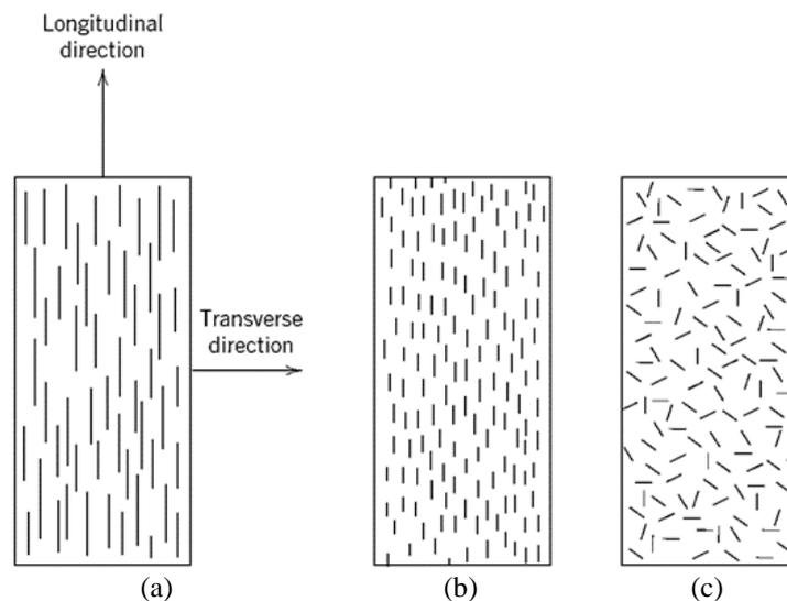
Fig. 11 - Schematic representation of the orientation of fiber-reinforced composite [37]
