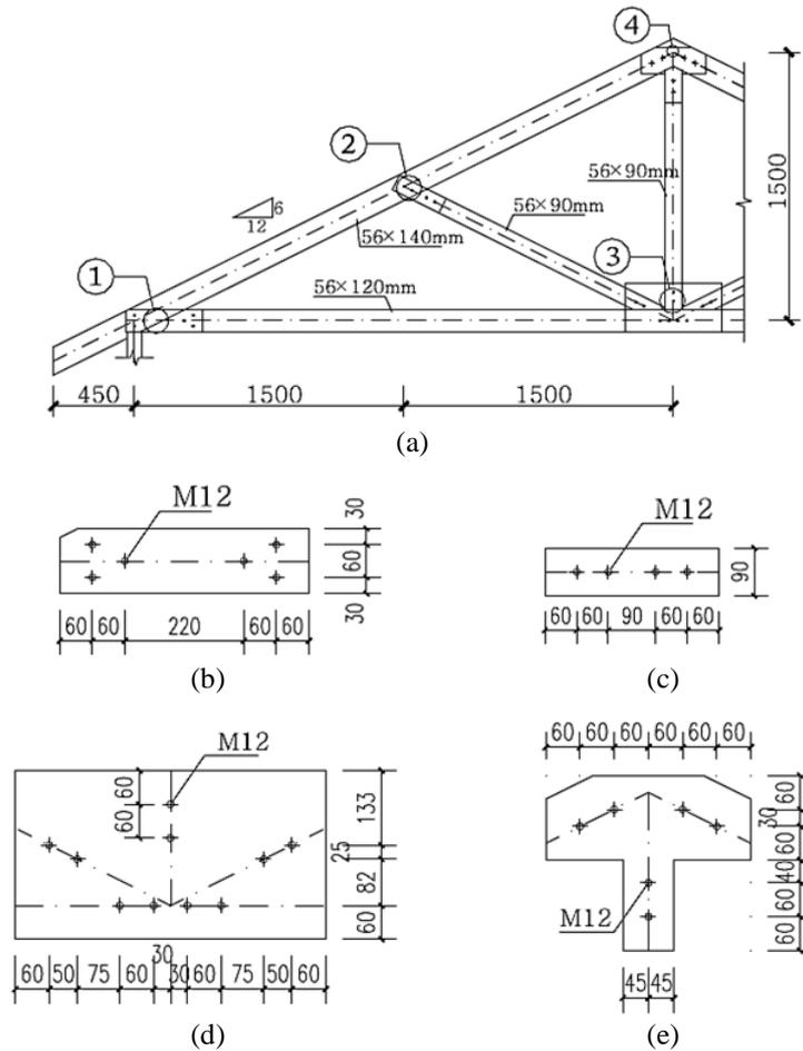
**Fig. 8 - The plate and bolt connection geometry for the glubam truss [17]**
