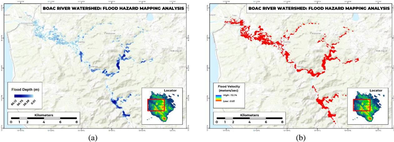
**Fig. 3 - Flood hazard analysis of Boac River watershed showing different simulations; (a) flood depth; (b) flood velocity**
