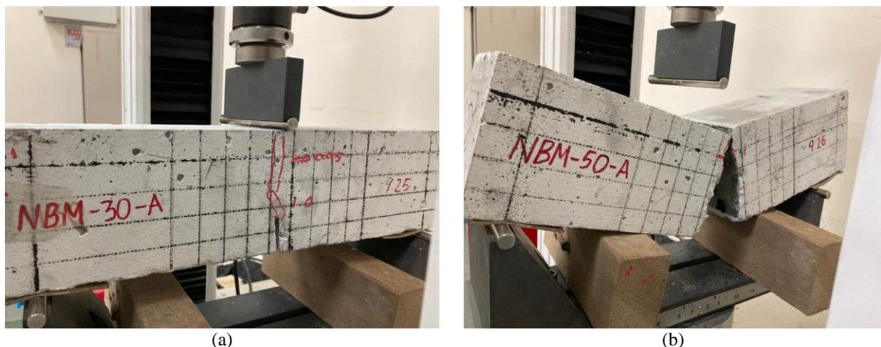
Fig. 2 - Mechanical testing set-up; (a) crack propagation marking; (b) a completely ruptured concrete beam specimen
