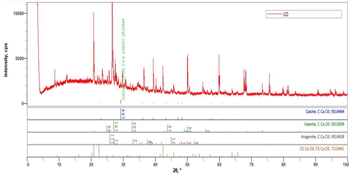
**Fig. 10 - X-ray diffraction of treated specimen**
