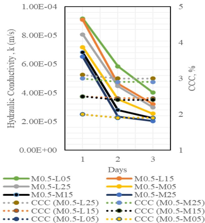
Fig. 7 - Hydraulic conductivity and calcium carbonate content (0.5M)
