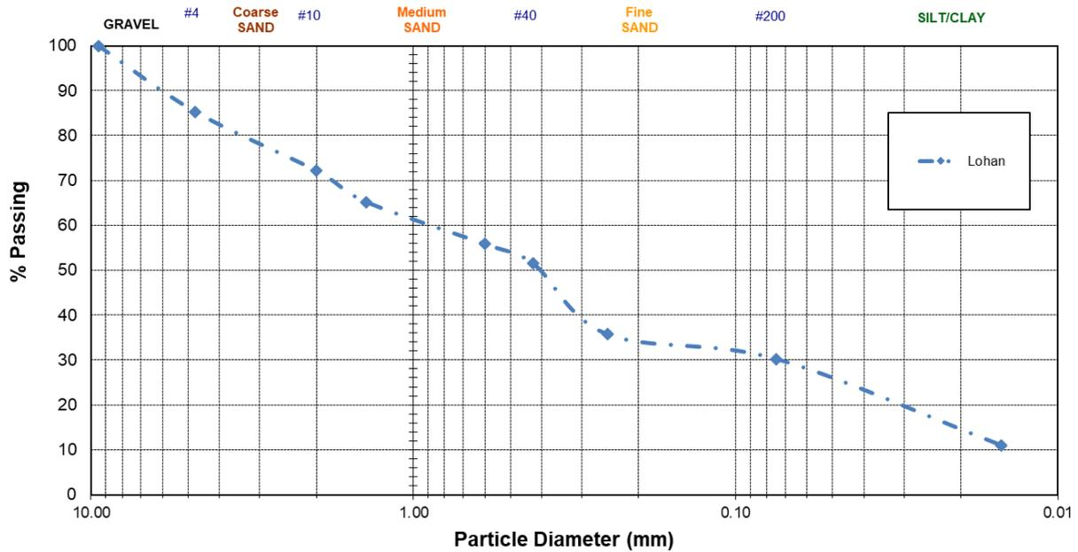
Fig 2 - Particle size distribution of Lohan Dam mine waste soil
