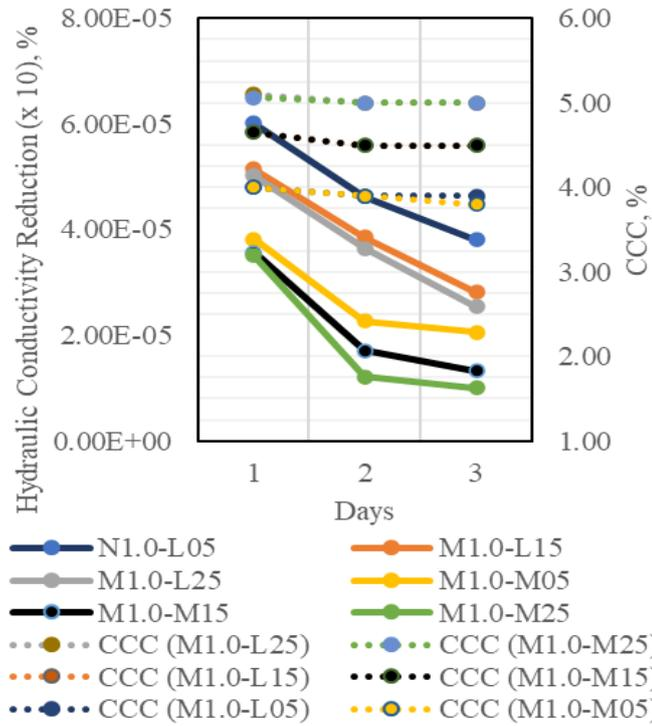
**Fig. 8 - Hydraulic conductivity and calcium carbonate content (1.0M)**
