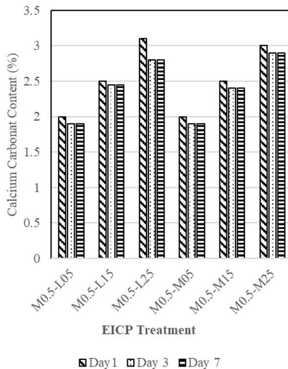
**Fig. 5 - Calcium carbonate content of treated Lohan soil (0.5M)**
