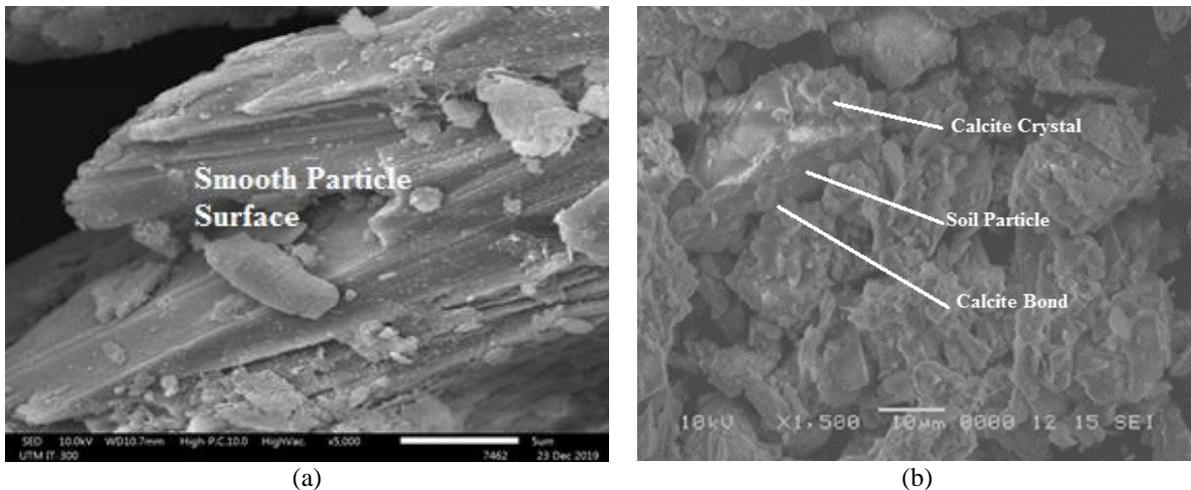
**Fig. 9 - (a) SEM of original specimen and; (b) SEM of treated specimen**
