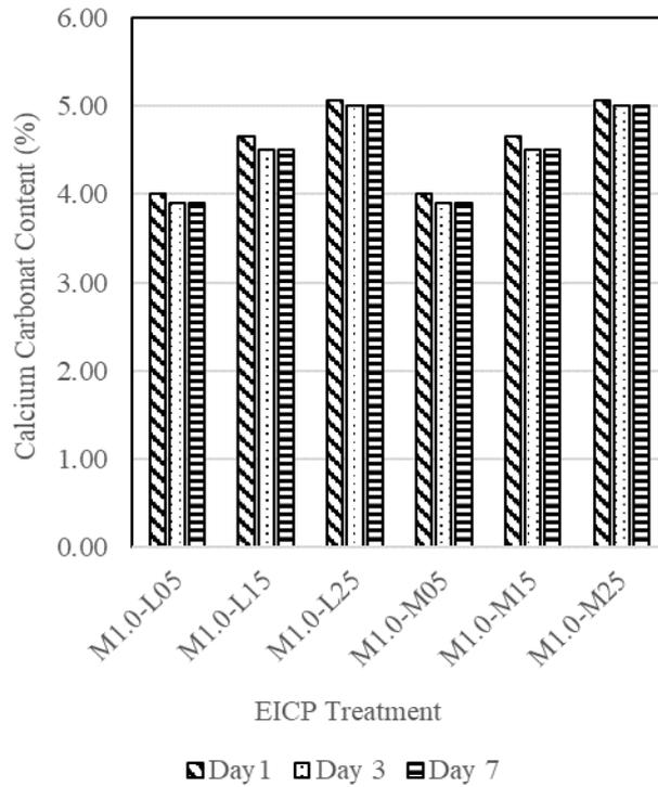
Fig. 6 - Calcium carbonate content of treated Lohan soil (1.0M)
