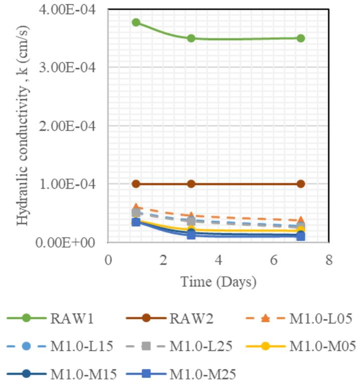
Fig. 4 - Hydraulic conductivity of Lohan soil (1.0 M)
