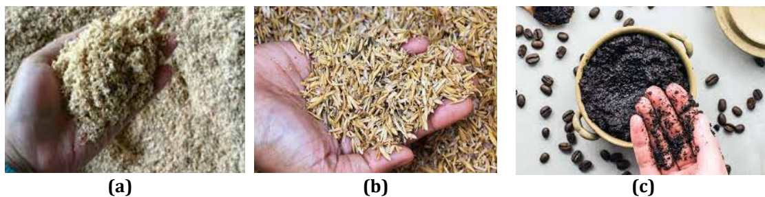
Fig. 1 Lignocellulosic substrate plant waste; (a) Sawdust; (b) Rice husks; (c) Coffee grounds
