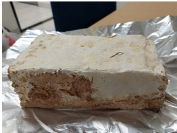
Fig. 16 Mycelium variation of sawdust after being in the oven at 80^{\circ}\text{C} for 60 minutes
