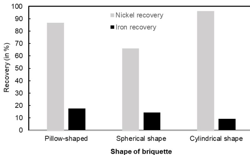
Fig. 6 Recovery value of each briquette shapes
