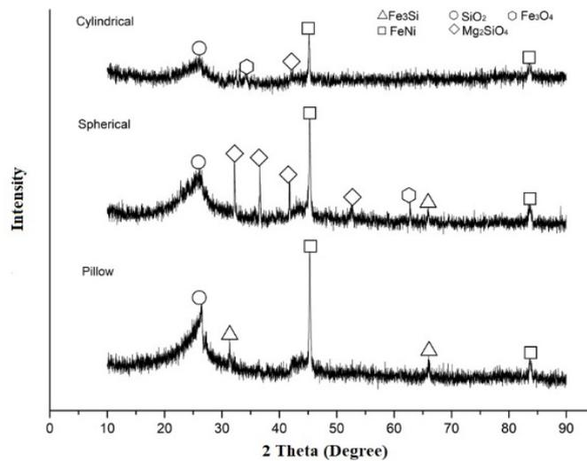
Fig. 7 Compounds are formed on each briquette shape
