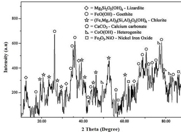
Fig. 1 XRD diffractogram of laterite nickel
