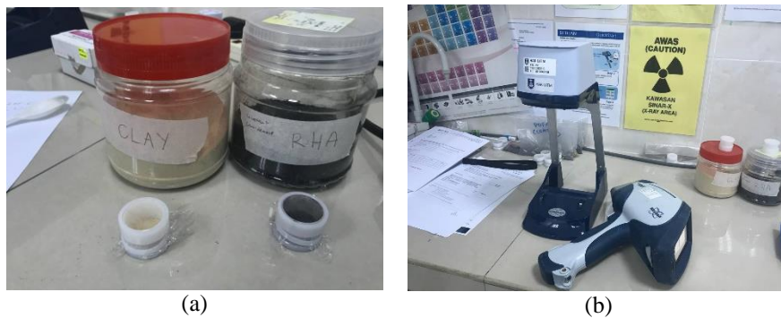
Fig. 2 - XRF test; (a) samples; (b) XRF analyzer
