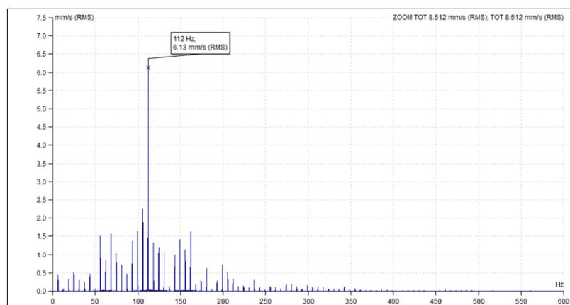
**Fig. 8 - Velocity spectrum of Motor DE Axial - highest peak plotted at 112 Hz**
