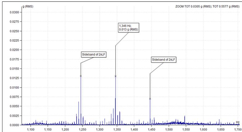
**Fig. 9 - Acceleration spectrum of Motor NDE Axial - Rotor Bar Frequency (RBF) with sideband of 2xLF**
