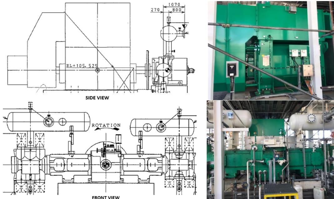
**Fig. 3 - Motor-compressor configuration**
