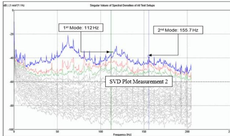
**Fig. 12 - SVD plot for Measurement 2**
