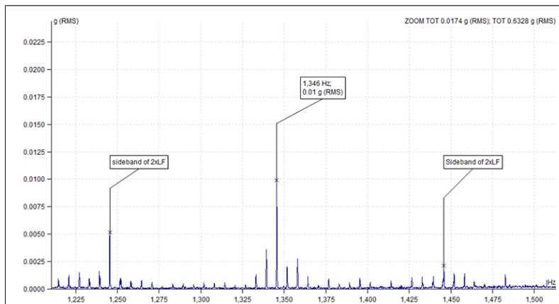
**Fig. 10 - Acceleration spectrum of Motor DE Axial - Rotor Bar Frequency (RBF) with sideband of 2xLF**
