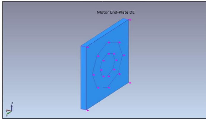
Fig. 6 - Geometry and DOF for Measurement 2
