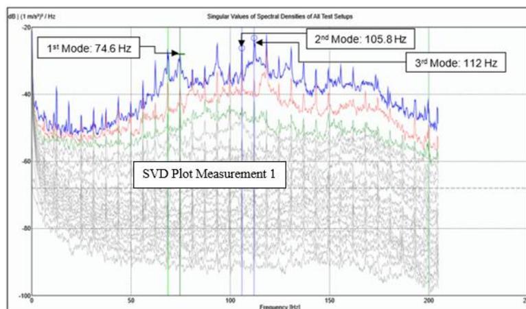
**Fig. 11 - SVD plot for Measurement 1**
