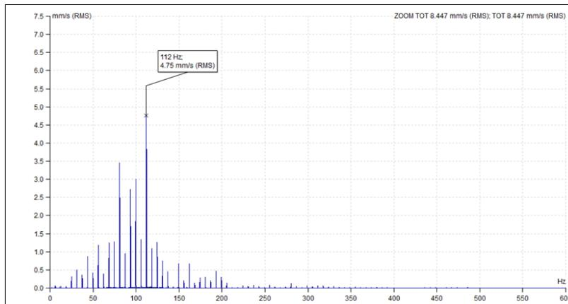
**Fig. 7 - Velocity spectrum of Motor NDE Axial - highest peak plotted at 112 Hz**
