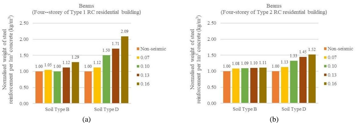
**Fig. 4 - Total steel reinforcement weight normalized to 1m<sup>3</sup> concrete for four storey RC residential building beams; (a) Type 1; (b) Type 2**
