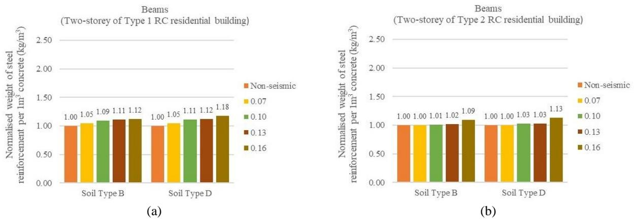
**Fig. 3 - Total steel reinforcement weight normalized to 1m<sup>3</sup> concrete for two storey RC residential building beams; (a) Type 1; (b) Type 2**
