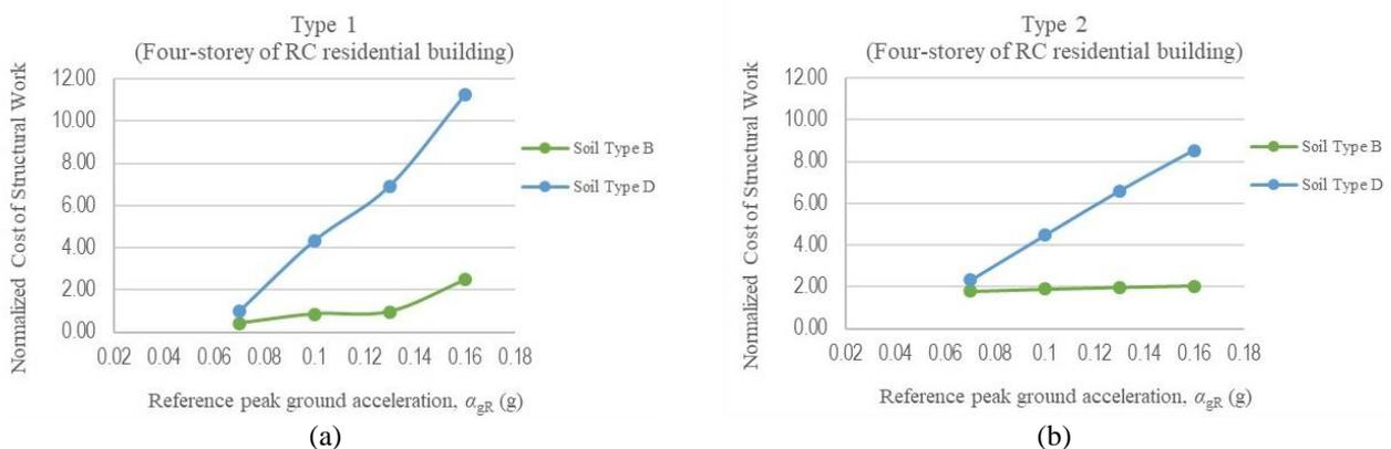
Fig. 8 - Normalized cost of structural works for four storey of RC residential building; (a) Type 1; (b) Type 2
