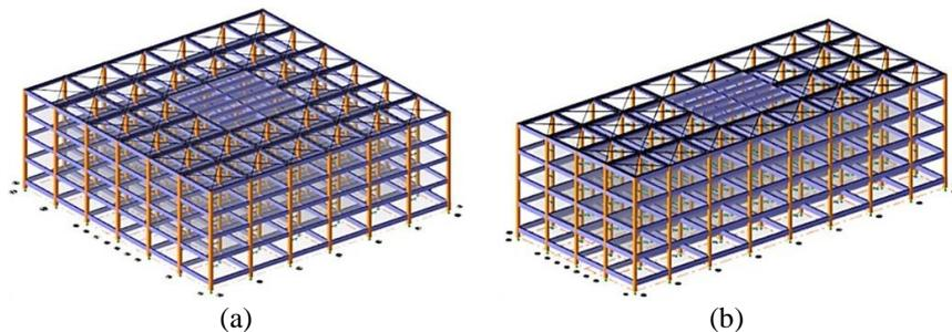
Fig. 2 - Four-storey RC residential building in 3D view; (a) Type 1; (b) Type 2
