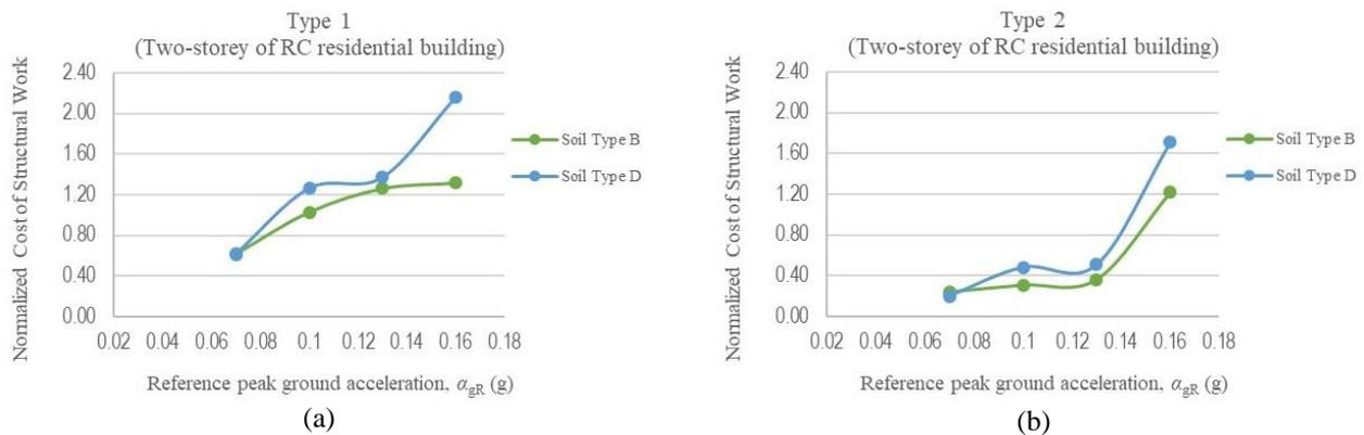
Fig. 7 - Normalized cost of structural works for two storey of RC residential building; (a) Type 1; (b) Type 2
