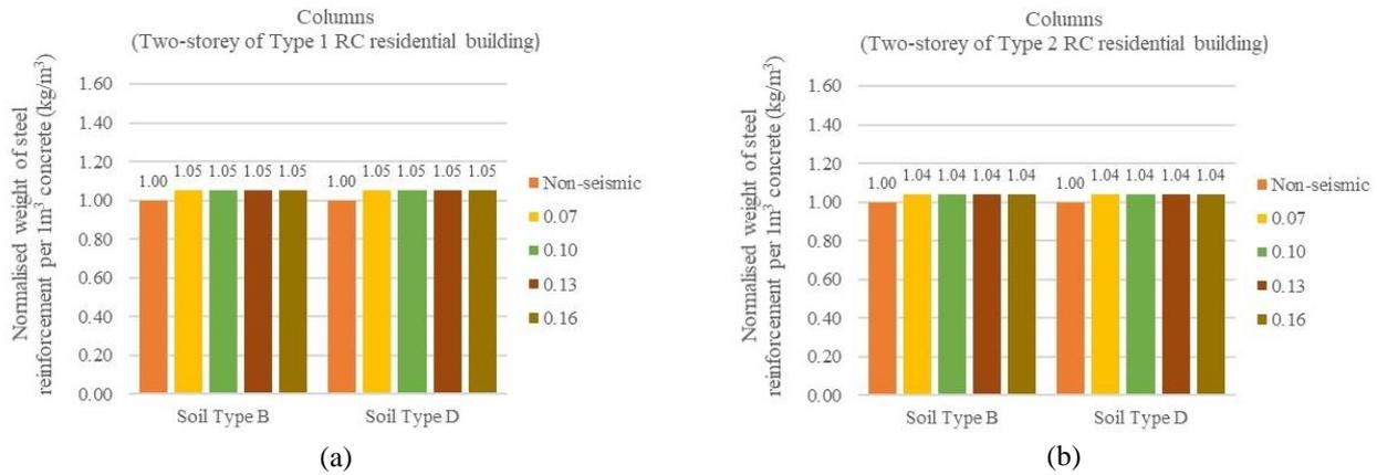
**Fig. 5 - Total steel reinforcement weight normalized to 1m<sup>3</sup> concrete for two storey RC residential building columns; (a) Type 1; (b) Type 2**
