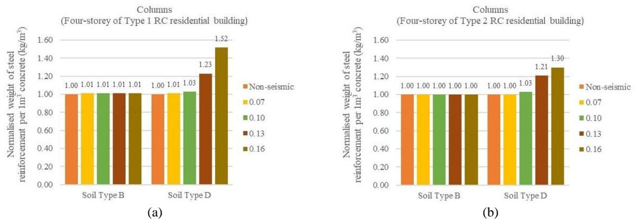
**Fig. 6 - Total steel reinforcement weight normalized to 1m<sup>3</sup> concrete for four storey RC residential building columns; (a) Type 1; (b) Type 2**
