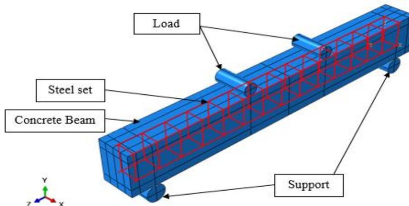
**Fig. 5 - The details of beam assembled**
