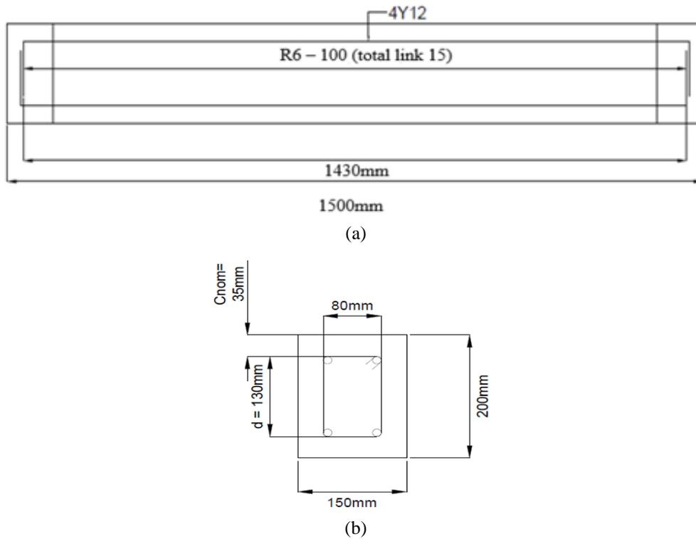
Fig. 2 - (a) Beam detailing; (b) beam cross section
