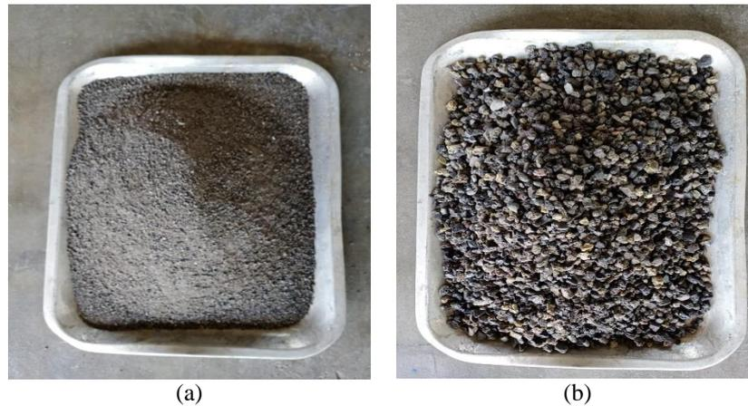
Fig. 1 - (a) Fine Coal Bottom Ash (FCBA); (b) Coarse Coal Bottom Ash (CCBA)
