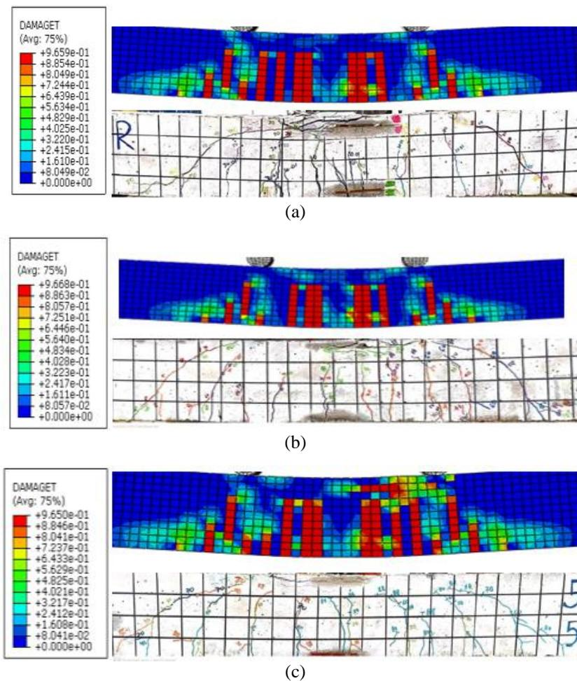
**Fig. 6 - (a) Control beam racking pattern; (b) 100% CCBA 100% FCBA cracking pattern; (c) 50% CCBA 50% FCBA cracking pattern**
