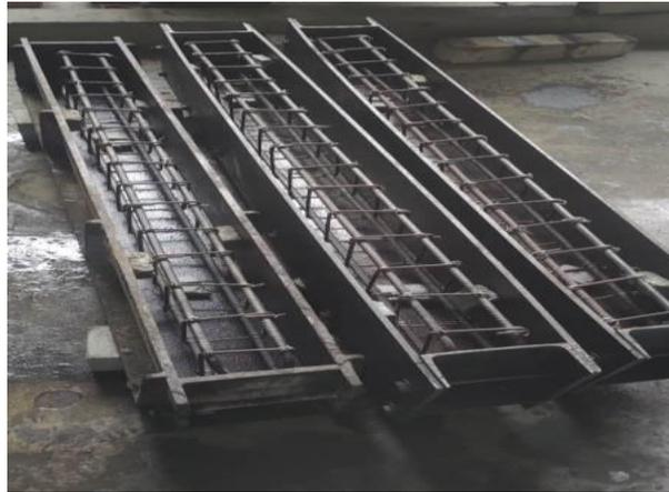
**Fig. 3 - Tied rebar in mould with 35mm concrete cover**
