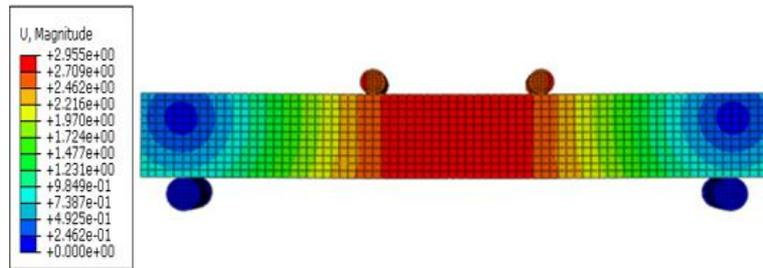
**Fig. 8 - Deflection of RC beams using FEA**
