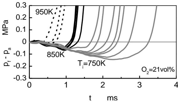
Fig. 4 Illustration of Ignition delay [2]
