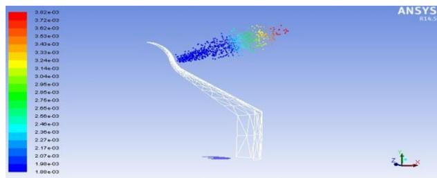
Fig. 11 The structure of the particle sprays penetration form at ambient pressure of 2 MPa with 1 spray nozzle.
