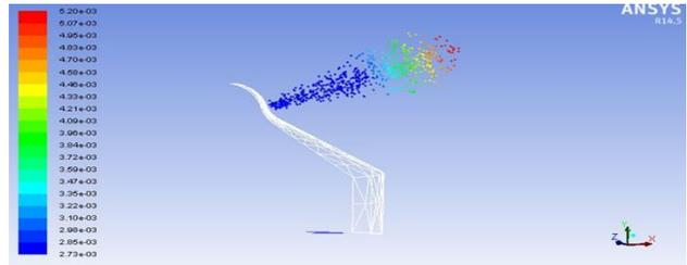
Fig. 7 The structure of the particle sprays penetration form at ambient pressure of 4 MPa with 1 spray nozzle.
