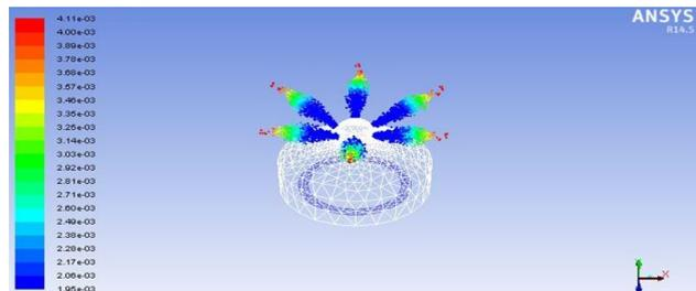
Fig. 10 The structure of the particle spray penetration form at ambient pressure of 3 MPa with 6 sprays nozzle.
