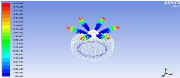
Fig. 12 The structure of the particle spray penetration form at ambient pressure of 4 MPa with 6 sprays nozzle.
