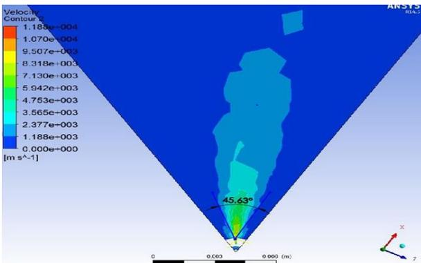
Fig. 13 Spray angle at 4MPa
