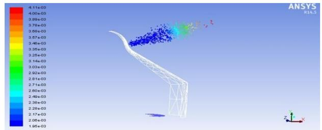
Fig. 9 The structure of the particle sprays penetration form at ambient pressure of 3 MPa with 1 spray nozzle.
