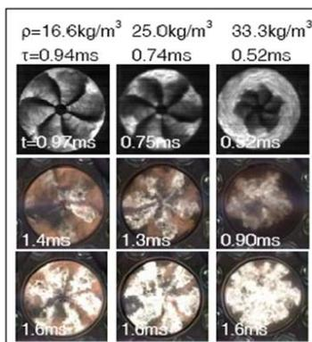
Fig. 5 Mixture formation and ignition [16].
