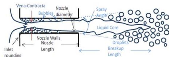
Fig. 3 Fuel atomization process [12].
