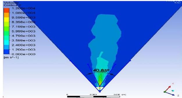
Fig. 15 Spray angle at 2MPa
