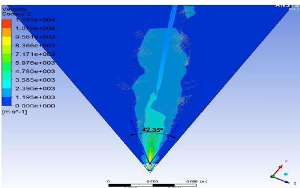
Fig. 14 Spray angle at 3MPa
