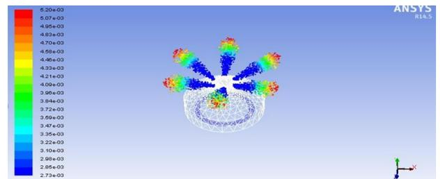
Fig. 8 The structure of the particle spray penetration form at ambient pressure of 4 MPa with 6 sprays nozzle.
