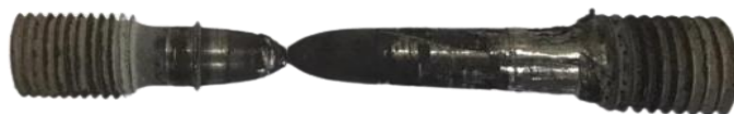
Fig. 5 - Rupture of P91 steel uniaxial round bar for the stress of unwelded 190 MPa at 31.33 hours
