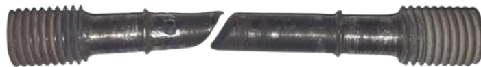
Fig. 4 - Rupture of P91 steel uniaxial round bar for the stress of welded 190 MPa at 50.60 hours
