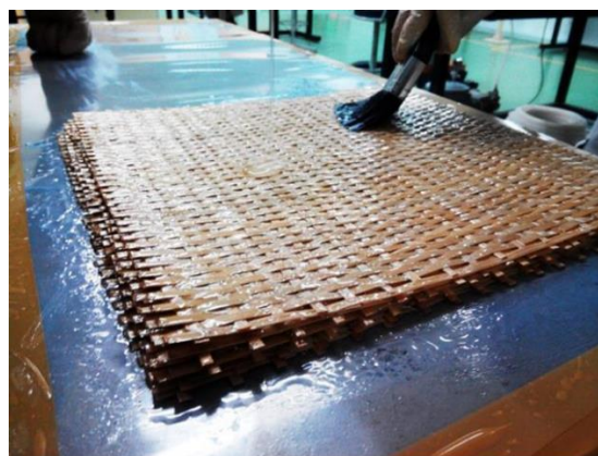
Fig. 3 - Hand lay-up technique of applying the UP onto each layer of woven bamboo and E-glass fibre
