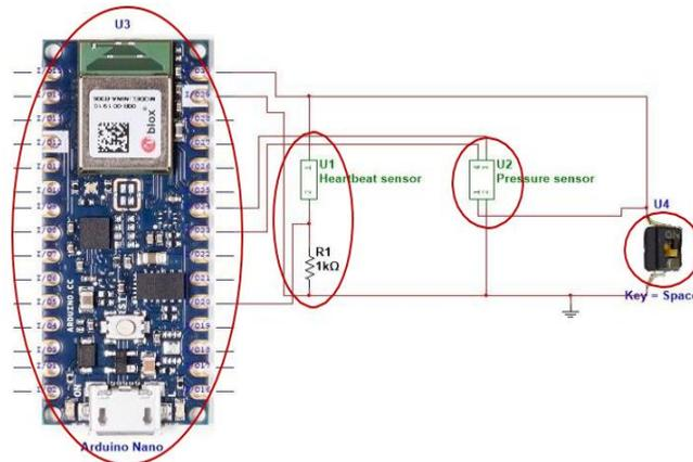
**Fig. 1 - Arduino connection with the sensors**
