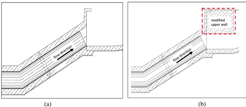
**Fig. 14 - Sketch of the configuration of the downstream channel (a) existing design, and; (b) modified design**
