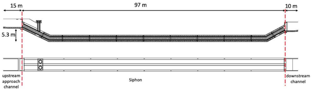
Fig. 2 - Long section of the Rambatan siphons (dimension in prototype scale)
