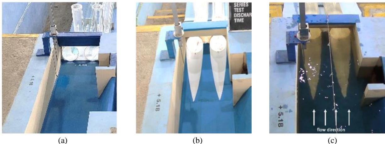
**Fig. 12 - Upstream part of the siphons (a) existing design; (b) modified design, and; (c) simulation with modified design (dimension in prototype scale)**
