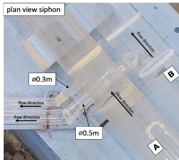
**Fig. 8 - Diversion pipe for the siphons (dimension in prototype scale)**
