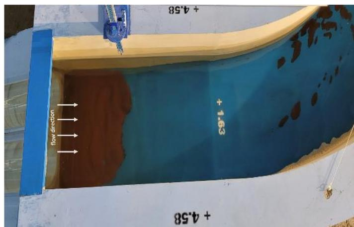
**Fig. 10 - Accumulated sediment remaining at the downstream channel with the existing design**
