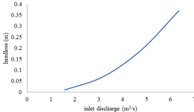
**Fig. 18 - Head loss for the siphons for different discharge values (dimension in prototype scale)**
