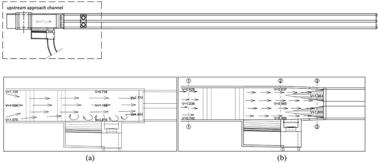
**Fig. 11 - Flow pattern of upstream channel with  $6.36 \text{ m}^3/\text{s}$  discharge (a) existing design, and; (b) modified design (dimension in prototype scale)**
