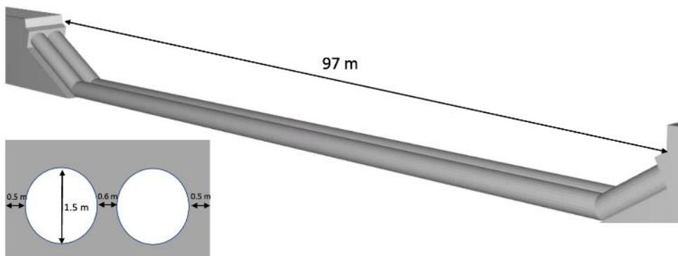
Fig. 3 - 3D view design of the Rambatan siphons (dimension prototype scale)
