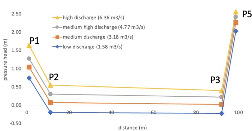
Fig. 17 - Piezometer results (dimension in prototype scale)
