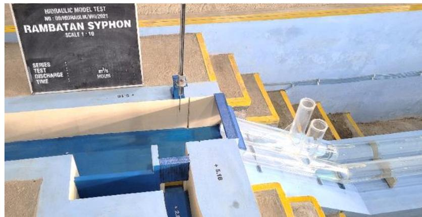
**Fig. 5 - Physical model of the Rambatan siphons**
