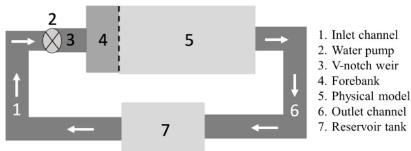
**Fig. 4 - Physical model configuration**
