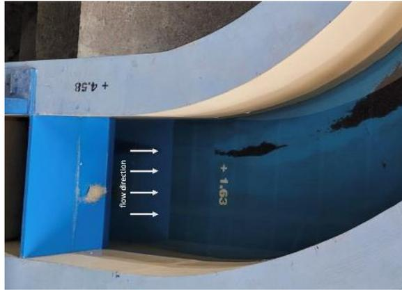
Fig. 15 - Accumulated sediment remaining at the downstream channel with the modified design
