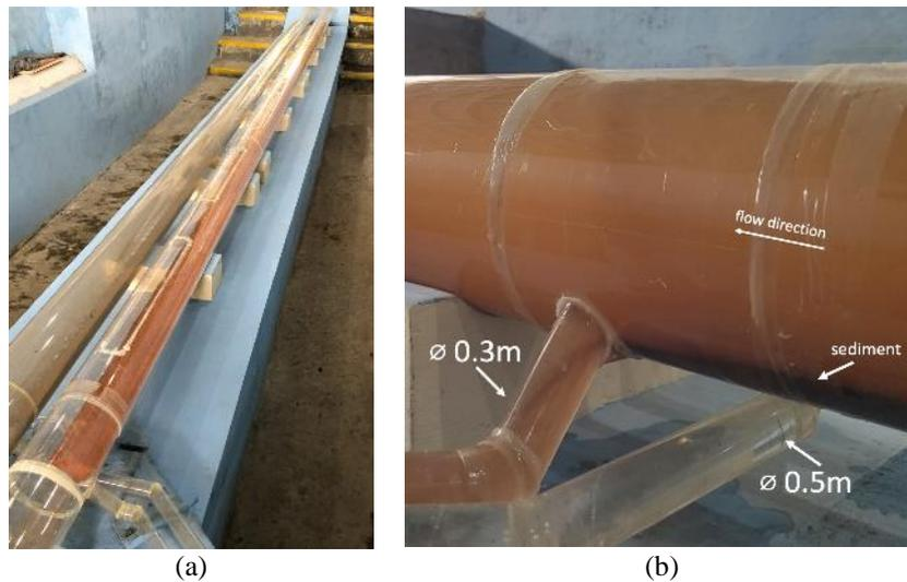
**Fig. 9 - (a) Before flushing simulation, and; (b) during flushing simulation to the 0.3 m pipe (dimension in prototype scale)**
