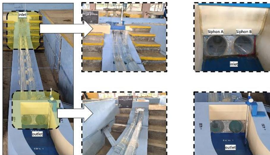
**Fig. 6 - Inlet and outlet configurations of the Rambatan siphons (physical model)**
