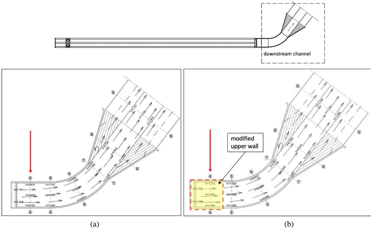
**Fig. 13 - Flow pattern of downstream channel with 6.36 m<sup>3</sup>/s discharge (a) existing design, and; (b) modified design (dimension in prototype scale)**
