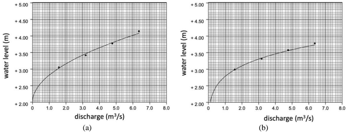
**Fig. 7 - Rating curve (a) upstream channel, and; (b) downstream channel (dimension in prototype scale)**
