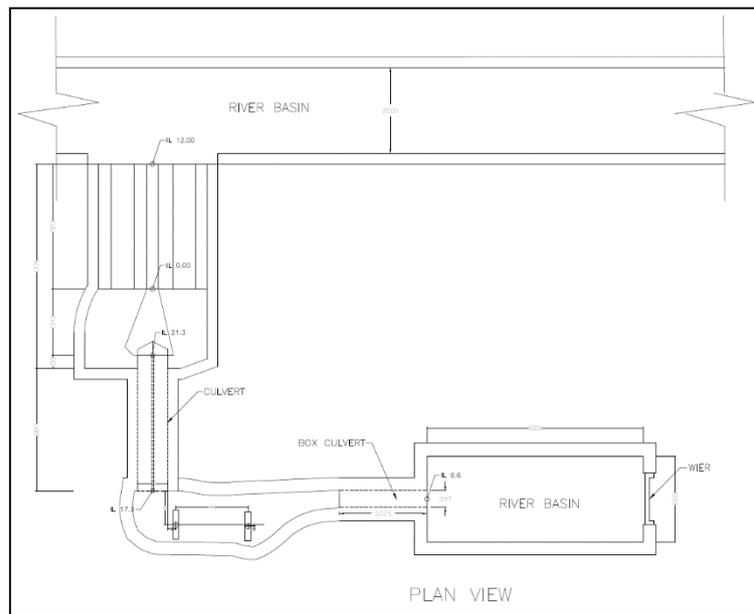
**Fig. 2 - Schematic plan view of the model setup**
