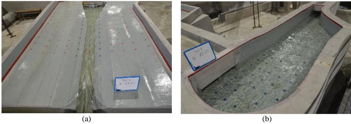
**Fig. 4 - Flow at discharge of 52 L/s at at (a) Sungai Bunus, and; (b) stilling basin (without piers)**
