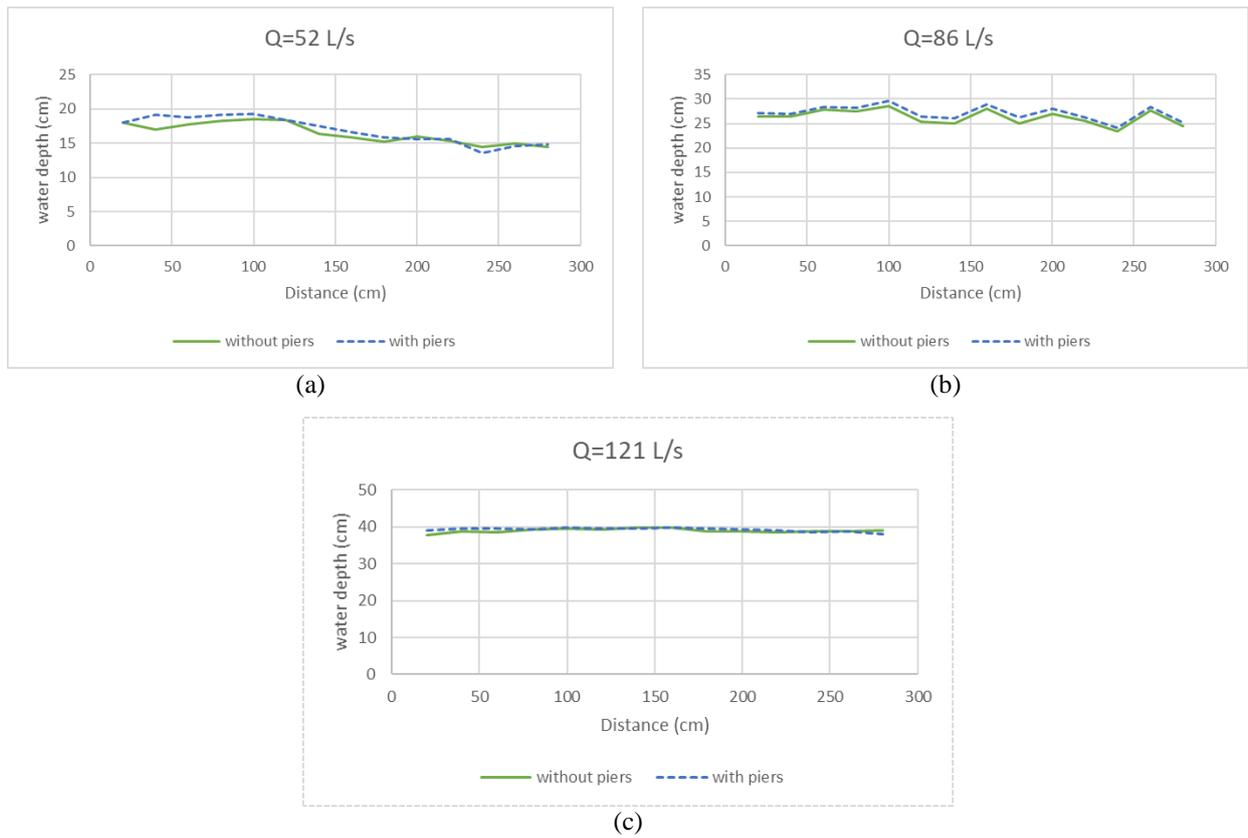
**Fig. 6 - Water surface height profiles for the stilling basin at discharge (a) 52 L/s; (b) 86 L/s; (c) 121 L/s**
