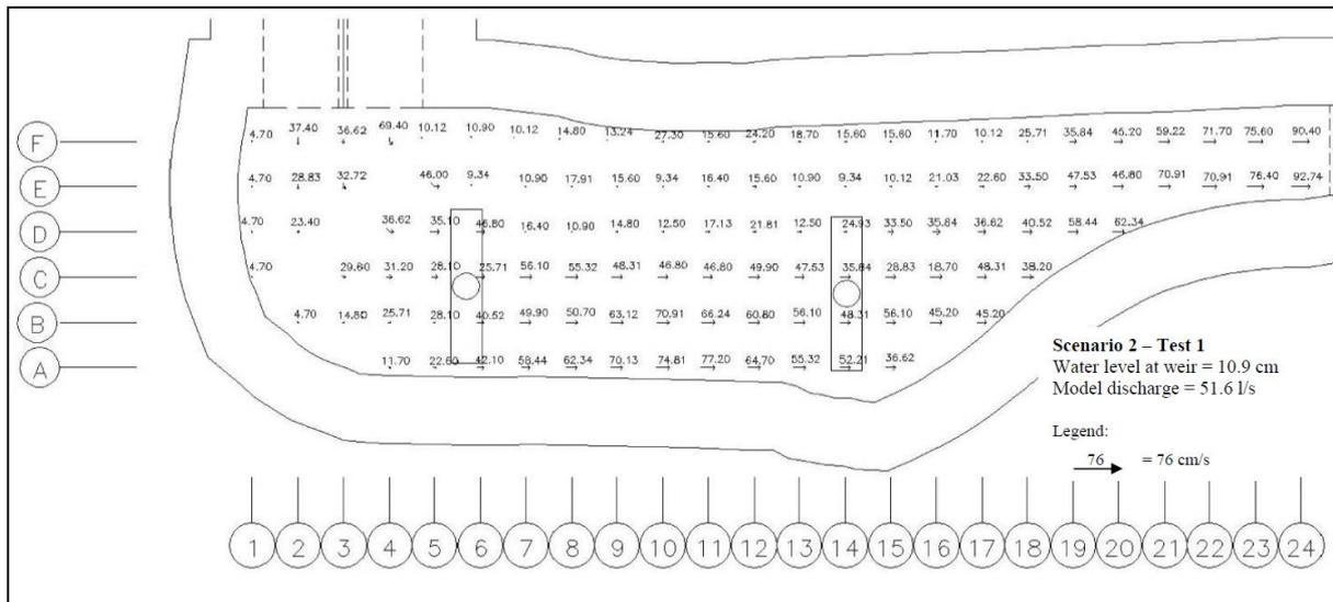
**Fig. 10 - Stilling basin velocity distribution maps for 51 L/s (with piers)**
