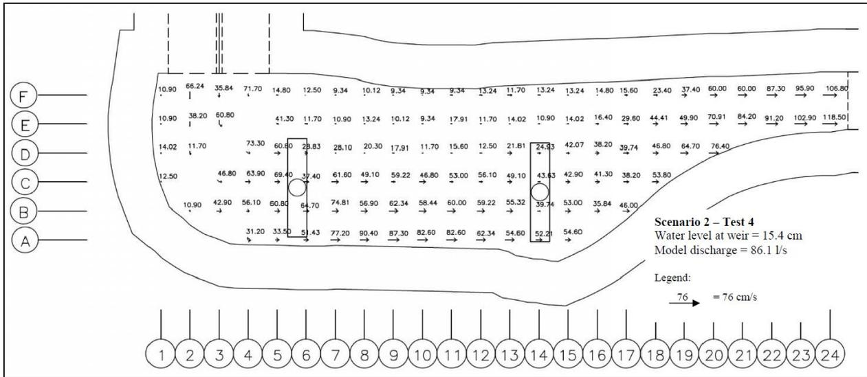
**Fig. 11 - Stilling basin velocity distribution maps for 86 L/s (with piers)**
