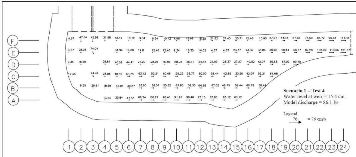
**Fig. 8 - Stilling Basin velocity distribution maps for 86 L/s (without piers)**
