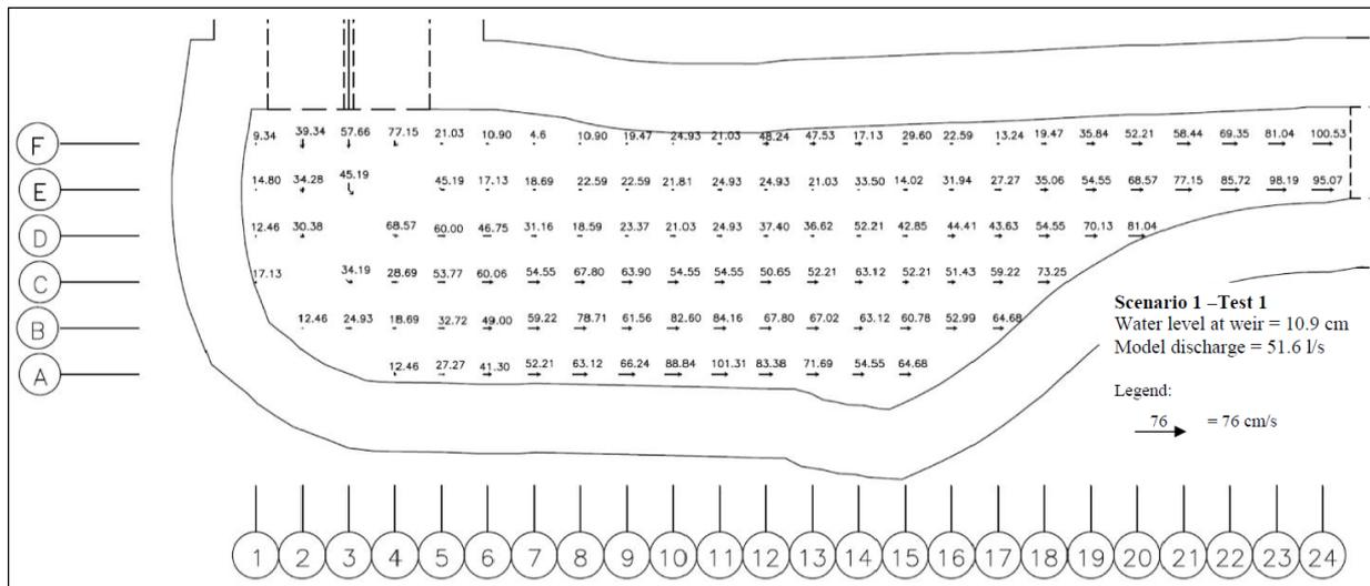
**Fig. 7 - Stilling basin velocity distribution maps for 51 L/s (without piers)**
