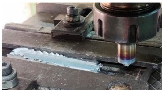
**Fig. 7** Flash generation during FS welding on the aluminium alloy plates
