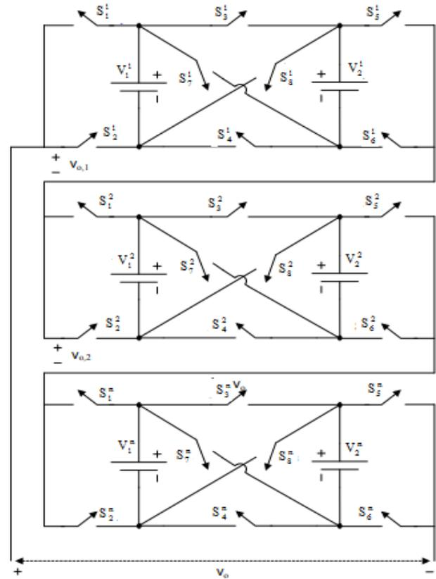
**Fig. 2** Proposed single phase cascaded multilevel inverter with 'n' units
