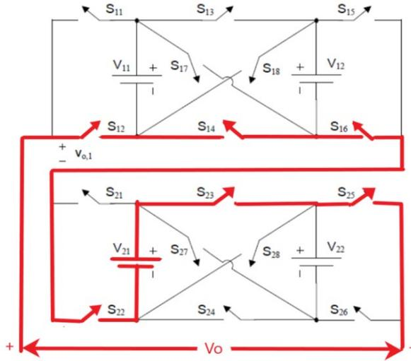
**Fig. 8** Current path of cross switched cascaded multilevel inverter for producing -150V
