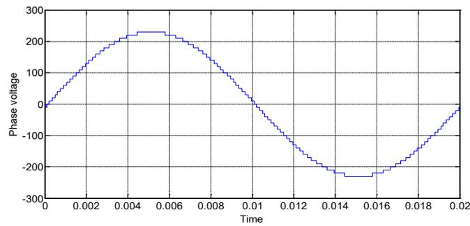
**Fig. 11** Output phase voltage of 49 level CSCMI (zoomed for one cycle)
