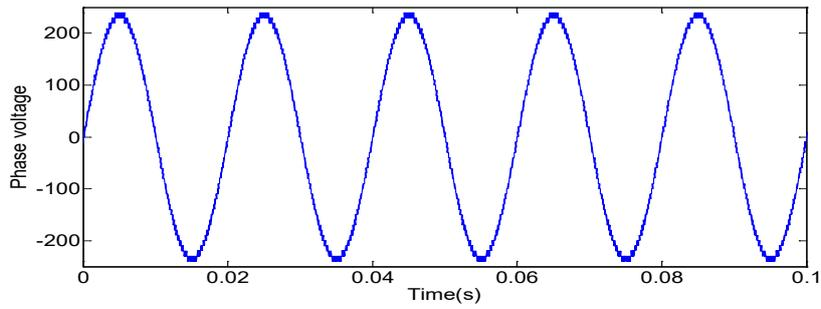
**Fig. 10** Output phase voltage of 49-level cross switched cascaded multilevel inverter.
