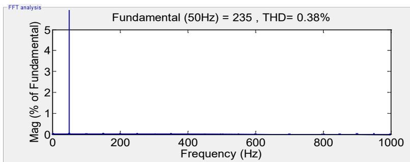
**Fig. 12** Total harmonic distortion of 49 level CSCMI output voltage
