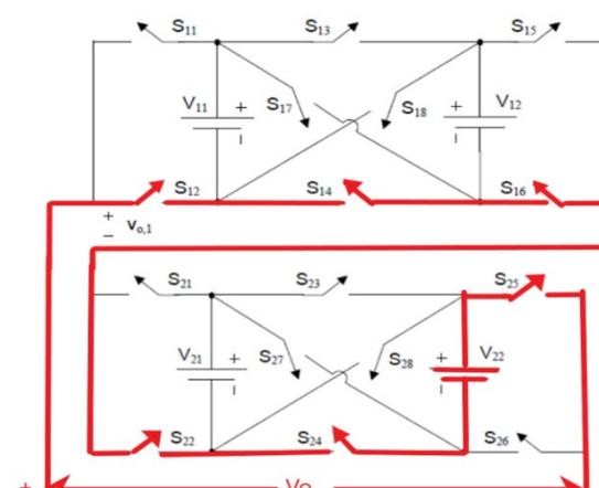
**Fig. 7** Current path of cross switched cascaded multilevel inverter for producing  $-50V$
