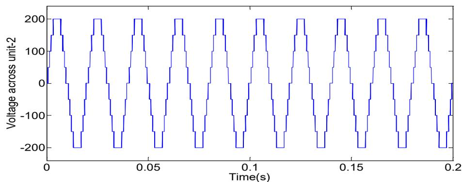
**Fig. 16** Voltage across unit 2
