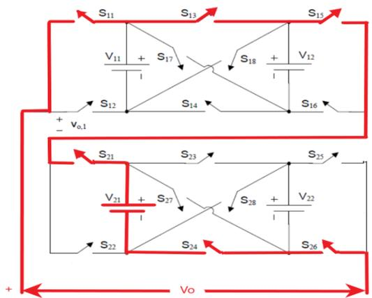
**Fig. 5** Current path of cross switched cascaded multilevel inverter for producing  $+150V$
