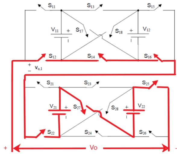
**Fig. 9** Current path of cross switched cascaded multilevel inverter for producing -200V
