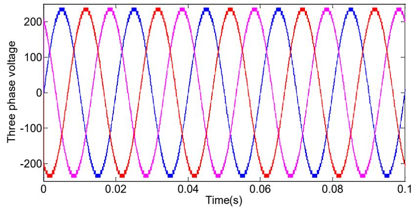
**Fig. 14** Three phase output voltage of 49 level CSCMI
