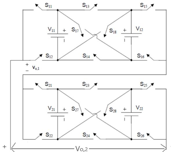
Fig. 3 Circuit diagram of 49-Level cross switched cascaded multilevel inverter
