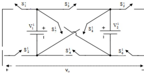
**Fig. 1** Proposed multilayer inverter's fundamental component
