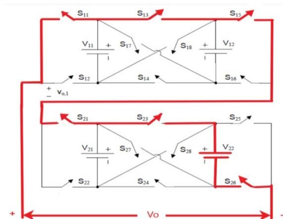
**Fig. 6** Current path of cross switched cascaded multilevel inverter for producing  $+50V$
