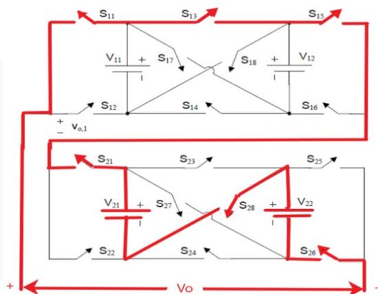
**Fig. 4** Current path of cross switched cascaded multilevel inverter for producing  $+200V$
