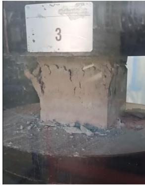
**Fig. 13 - The collapse mechanism of FC-GCW**
