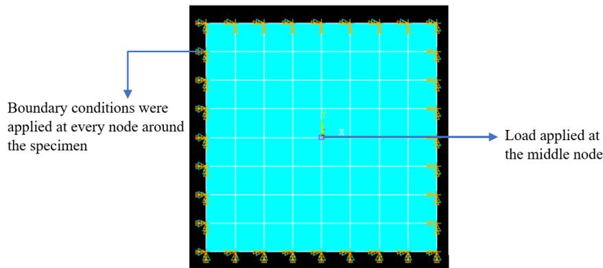
**Fig. 1 - Meshing element of the modelled specimen with boundary conditions**
