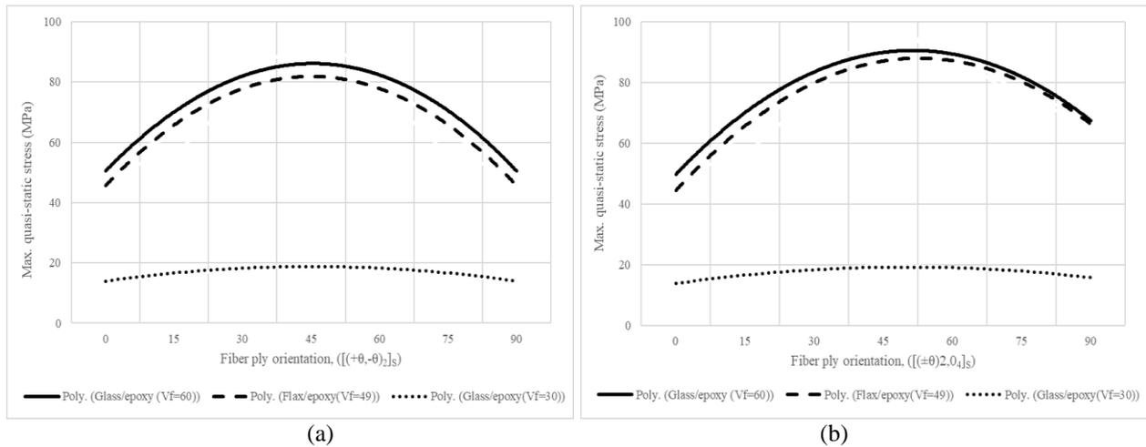
**Fig. 2 - Graph of maximum Quasi-static stress against fibre ply orientation of (a)  $[(+\theta, -\theta)_2]_s$  and (b)  $[(\pm\theta)_2, 0_4]_s$  for Glass/Epoxy (Vf = 60% and Vf = 30%) and flax/epoxy (Vf = 43%)**
