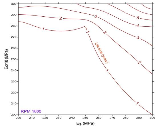
Fig. 5 Lifetime based on the ( $E_c$ ), ( $E_s$ ), and rpm=1800
