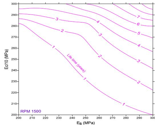
Fig. 4 Lifetime based on the ( $E_c$ ), ( $E_s$ ), and rpm=1500
