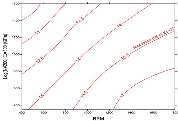
Fig. 6 Lifetime based on the speed and Log (N) for ( $E_s$ ) = 300 and ( $E_c$ ) = 20 GPa
