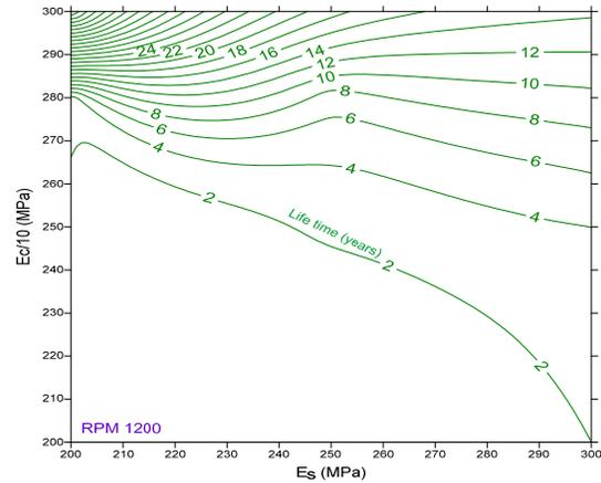
Fig. 3 Lifetime based on the ( $E_c$ ), ( $E_s$ ), and rpm=1200
