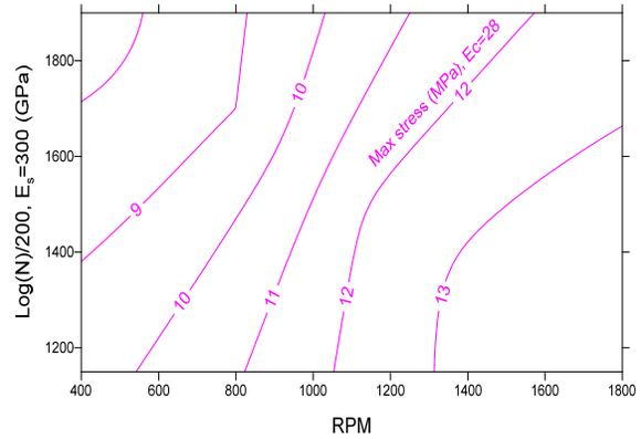
Fig. 8 Lifetime based on the speed and Log (N) for ( $E_s$ ) = 300 and ( $E_c$ ) = 28 GPa
