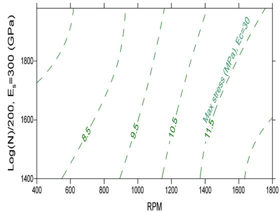
Fig. 9 Lifetime based on the speed and Log (N) for ( $E_s$ ) = 300 and ( $E_c$ ) = 30 GPa
