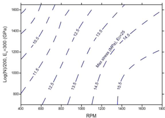
Fig. 7 Lifetime based on the speed and Log (N) for ( $E_s$ ) = 300 and ( $E_c$ ) = 25 GPa
