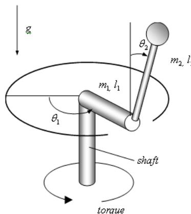
Fig. 1 Simplified rotary inverted pendulum schematic [22]
