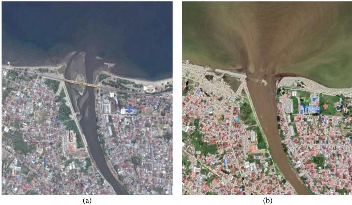
Fig. 2 - Situation of bed morphology in Palu Estuary (a) before before 2018 tsunami, and; (b) after 2018 tsunami
