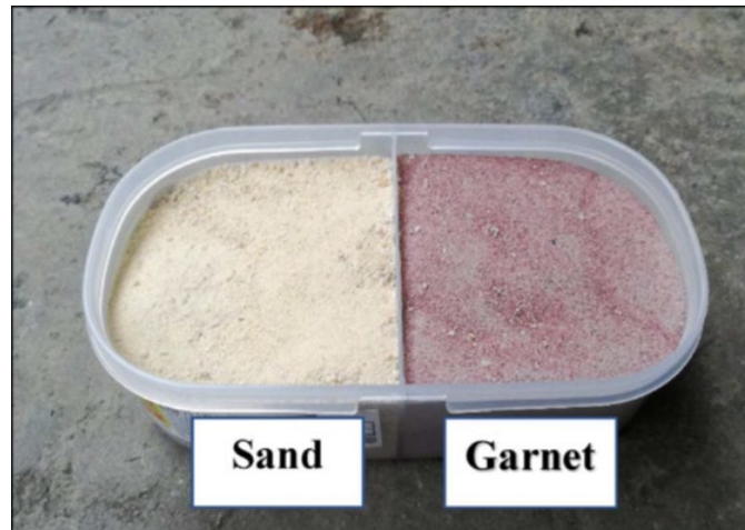
Fig. 2 - Appearance of fine aggregates (sand and garnet) used in the concrete production [8]
