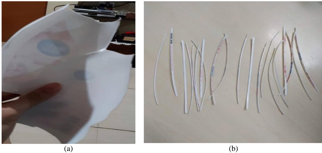
Fig. 2 - (a) Recycled HDPE Plastic; (b) recycled HDPE MFF after placed in shredder machine
