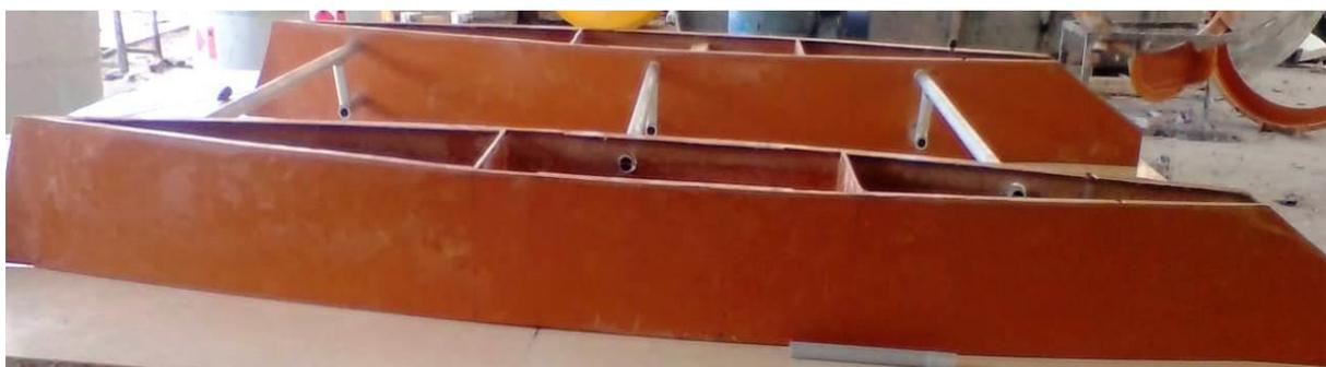
Fig. 3 - Moulded hull structure
