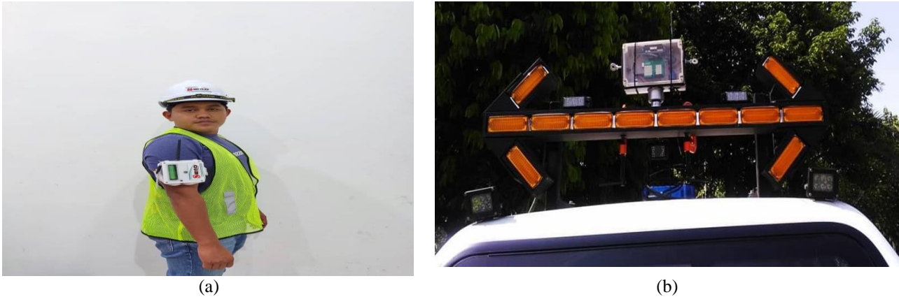
Fig. 3 - (a) Receiver and vibrator motor position; (b) Transmitter position
